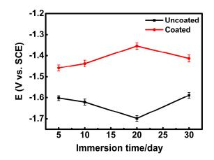
**Figure 11.** The evolution of open circuit potentials for the uncoated and the coated samples after immersion for 30 days.
