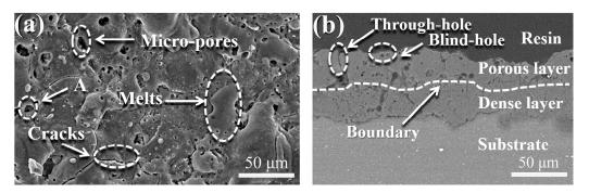
Figure 1. (a) Surface and (b) cross-sectional morphologies of micro-arc oxidation (MAO) coating.
