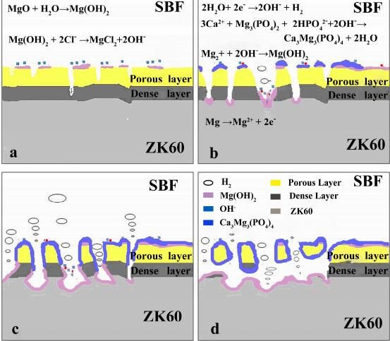
**Figure 13.** Degradation models of the MAO coated samples upon immersion in the SBF: (**a**) surface corrosion stage, (**b**) micro-pore enlargement stage, (**c**) coating degradation stage, and (**d**) coating decomposition stage.
