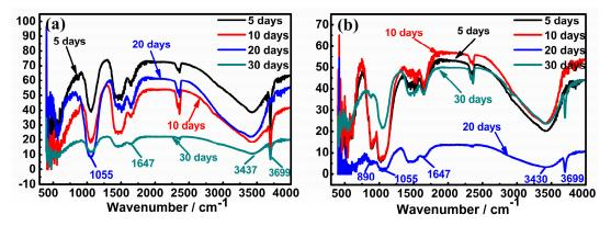
**Figure 8.** Fourier transform infrared spectroscopy (FTIR) of corrosion products on samples: (a) uncoated (b) MAO coated.
