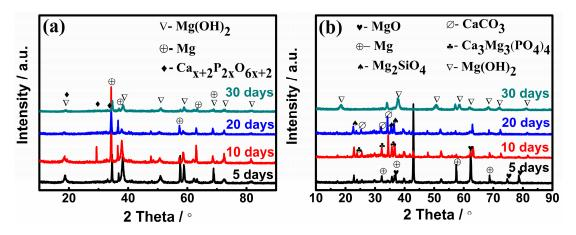
**Figure 7.** XRD patterns of (**a**) the uncoated and (**b**) the MAO coated samples after immersion for 30 days.
