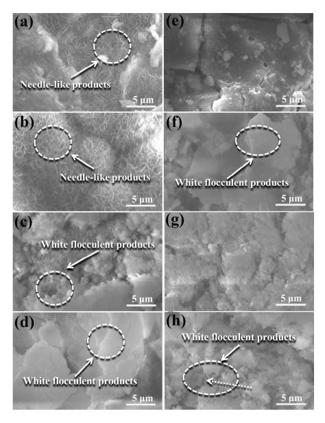
**Figure 6.** Morphologies of the uncoated and coated samples after immersion for 30 days: (**a**) 5 days, (**b**) 10 days, (**c**) 20 days, and (**d**) 30 days for uncoated sample, and (**e**) 5 days, (**f**) 10 days, (**g**) 20 days, and (**h**) 30 days for MAO coated sample, respectively.
