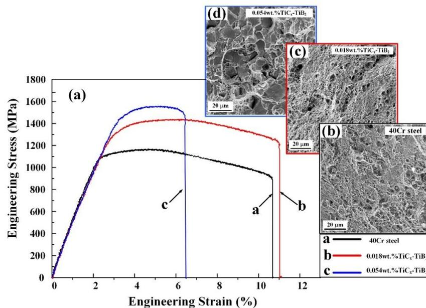
**Figure 7.** The tensile engineering stress-strain curves of steels with different  $\text{TiC}_x\text{-TiB}_2$  nanoparticles content in (a), and the corresponding fracture surfaces in (b–d).
