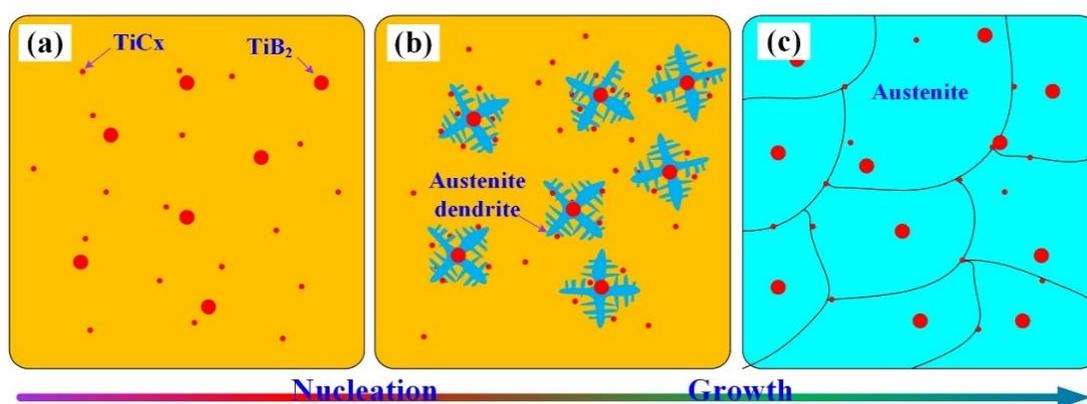
**Figure 6.** The effect of  $TiC_x-TiB_2$  nanoparticles on the refinement of austenite. (a) Nanoparticles in molten steel; (b) Nucleation and growth of austenite; (c) Nanoparticles in austenite.
