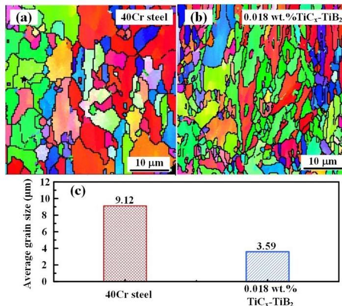
Figure 4. EBSD images of steels with  $\text{TiC}_x\text{-TiB}_2$  particles contents of 0 wt.% (a) and 0.018 wt.% (b) after heat treatment. (c) shows the average grain size of (a,b).
