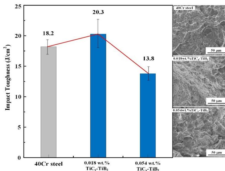
**Figure 9.** Impact toughness of steels with different contents of  $\text{TiC}_x\text{-TiB}_2$  nanoparticles and the corresponding impact fracture surfaces.
