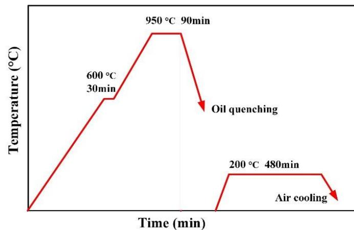
Figure 1. Heat treatment process diagram for cast steels.
