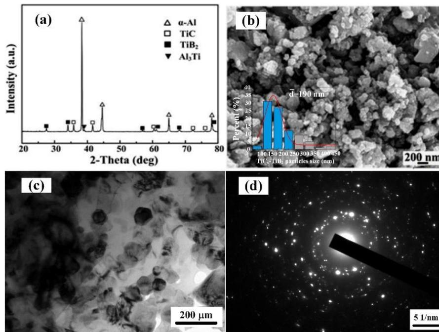
**Figure 2.** (a) XRD pattern of nano-sized TiC<sub>x</sub>-TiB<sub>2</sub>/Al master alloy, (b) morphologies and sizes analysis of the nano-sized TiC<sub>x</sub>-TiB<sub>2</sub> particles in the nano-sized TiC<sub>x</sub>-TiB<sub>2</sub>/Al master alloy. TEM images (c) and electron diffraction patterns (d) of the nano-sized TiC<sub>x</sub>-TiB<sub>2</sub>/Al master alloy.
