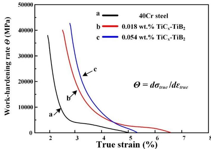
**Figure 8.** The corresponding work-hardening rate-true strain curves that were obtained from the tensile curve.
