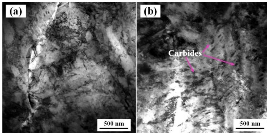
**Figure 5.** TEM images of steels without nano-sized  $TiC_x-TiB_2$  particles (a) and steels with 0.018 wt.%  $TiC_x-TiB_2$  nanoparticles (b).
