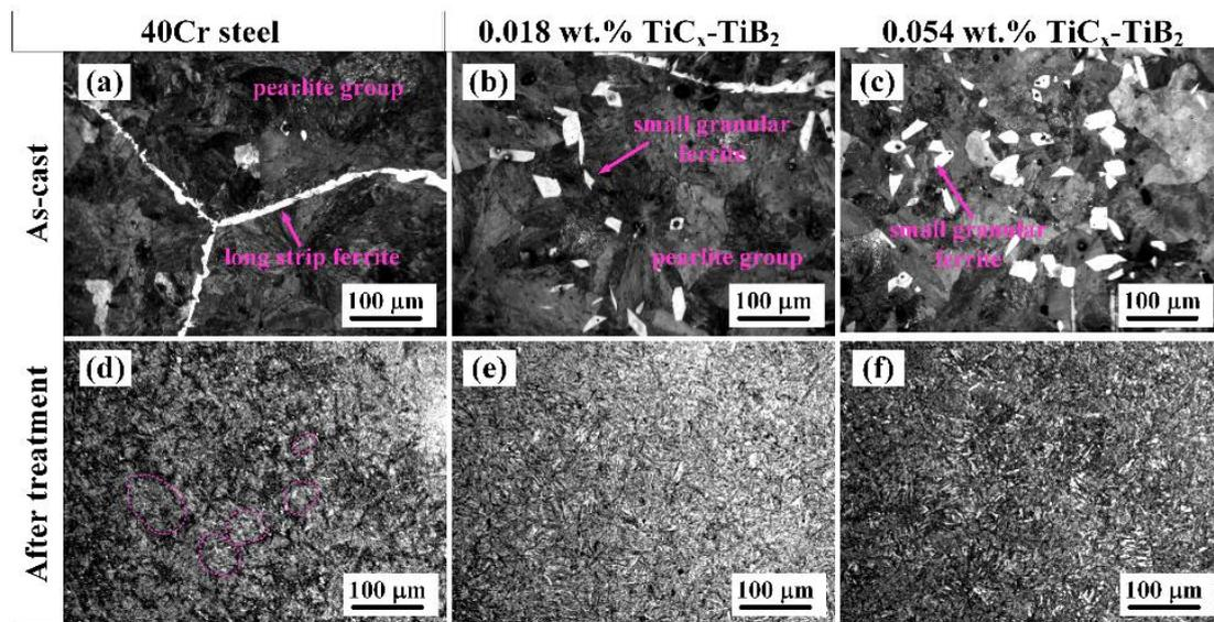
Figure 3. OM images of the as-cast steels (a–c), and steels after heat treatment (d–f).
