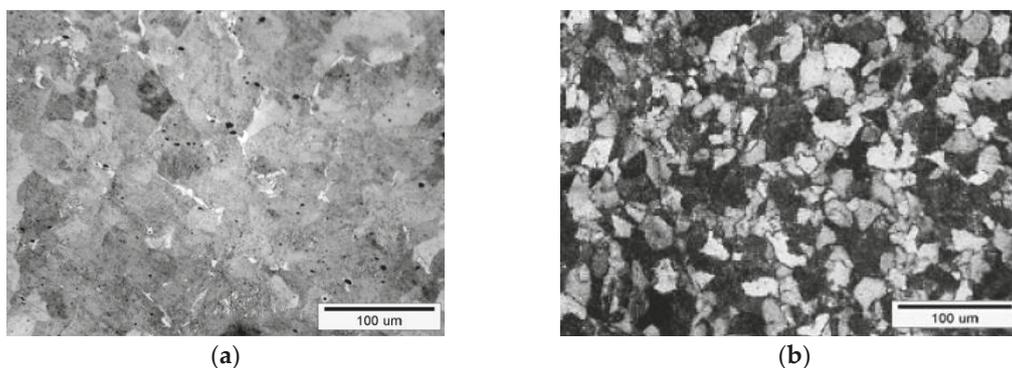
**Figure 2.** Optical microstructure of the tested steels: (a) C70S6; (b) 36MnVS4.
