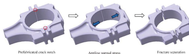
Figure 1. Connecting rod fracture-split process.
