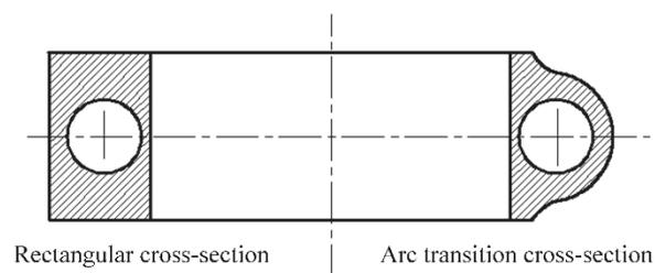
**Figure 12.** Cross-section design.
