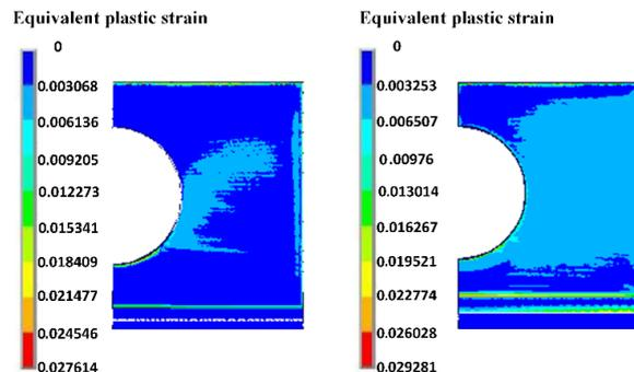
Figure 7. The plastic strain of the fracture surface: (a) C70S6; (b) 36MnVS4.
