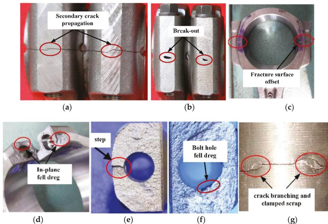
**Figure 11.** Fracture-splitting defects of the 36MnVS4 connecting rod: (a) crack bifurcation; (b) break-out; (c) fracture surface offset; (d) in-plane fell dregs; (e) step; (f) bolt hole fell dregs; (g) crack branching and clamped scrap.
