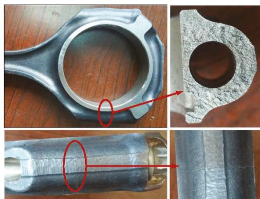
**Figure 13.** Experimental results of connecting rod fracture-split.
