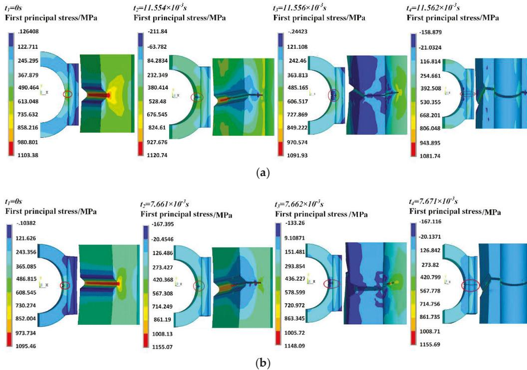
Figure 6. The first principal stress distribution of the connecting rods: (a) C70S6; (b) 36MnVS4.
