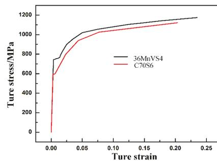
Figure 3. Tensile test curves.
