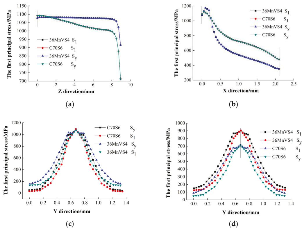
Figure 9. The stress of the feature lines in crack initiation: (a) Line 1; (b) Line 2; (c) Line 3; (d) Line 4.
