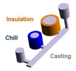
Figure 2. Cylindrical castings with the insulation and chill.
