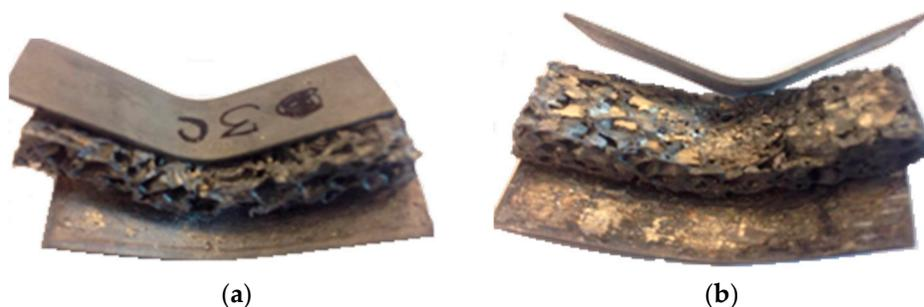
**Figure 11.** Representative post-three-point bending test delaminated specimens (specimen dimensions: 60 mm × 20 mm × 11.4 mm). (a) Brazed using Al-Cu-Mg and (b) brazed using Al-Si-Mg-Ti brazing alloy.
