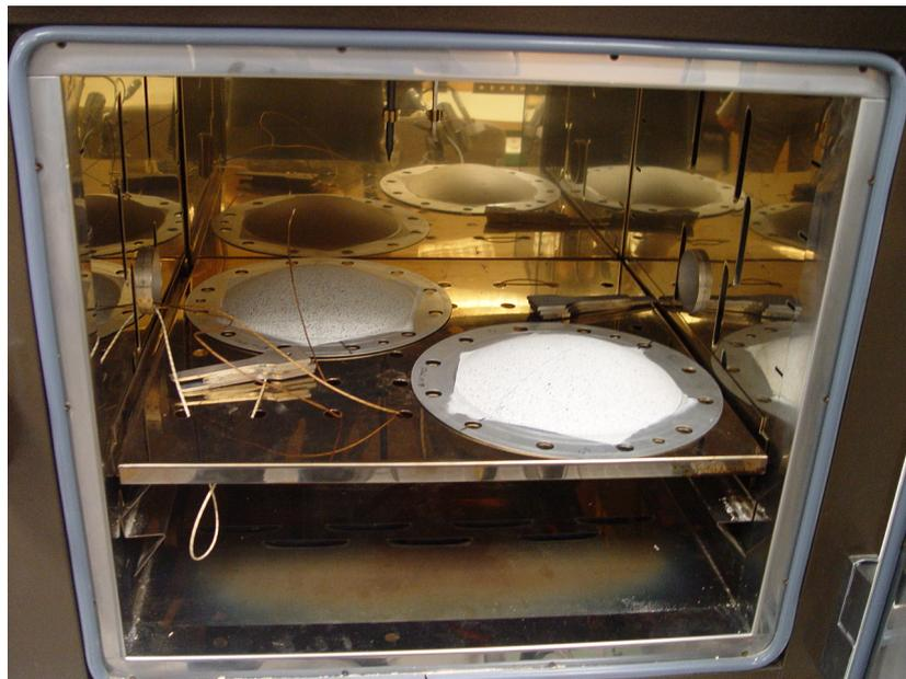
**Figure 3.** Thermal treatment of bulged specimen.
