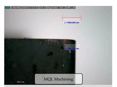
Figure 6. No built-up edge (Experiment no-11).
