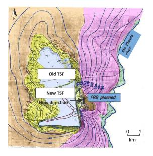
Figure 2. Hydrogeological map of the tailings storage facility site with hydroisohypses of the aquifer.
