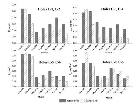
**Figure 8.** Uranium content in groundwater at PRB site: before PRB (monitoring hole C-1, C-3, C-5, C-7); after PRB (monitoring hole C-2, C-4, C-6, C-8) (Figure 7).
