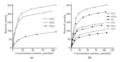
**Figure 5.** (a) Removal of U(VI) by different types of  $Fe^0$ ; (b) Effect of selected ligands (FA, EDTA, NTA, EDA, and Na<sub>2</sub>CO<sub>3</sub>) on the U(VI) removal by ZVI1.
