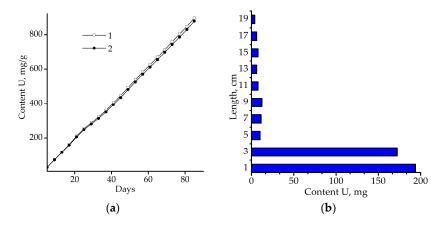
**Figure 6.** (a) Uranium released from contaminated water in column with ZVI2 and sand: 1—total uranium in the influent; 2—total released uranium; (b) Distribution of uranium in the reactive media in the column.
