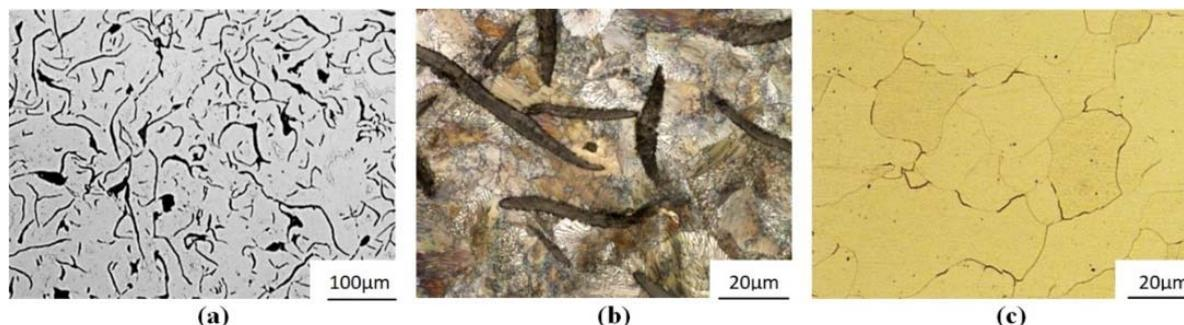
**Figure 3.** Alloys: (a) No. 6 cast iron GJL-300—eutectic colonies of IA3/4 graphite; (b) No. 6 cast iron GJL-300—pearlitic matrix, straight graphite IA3/4 ( $S_C = 0.98$ ) and (c) No 7—ferritic structure of Armco iron; (a) unetched; (b,c) etched with Mi1Fe.
