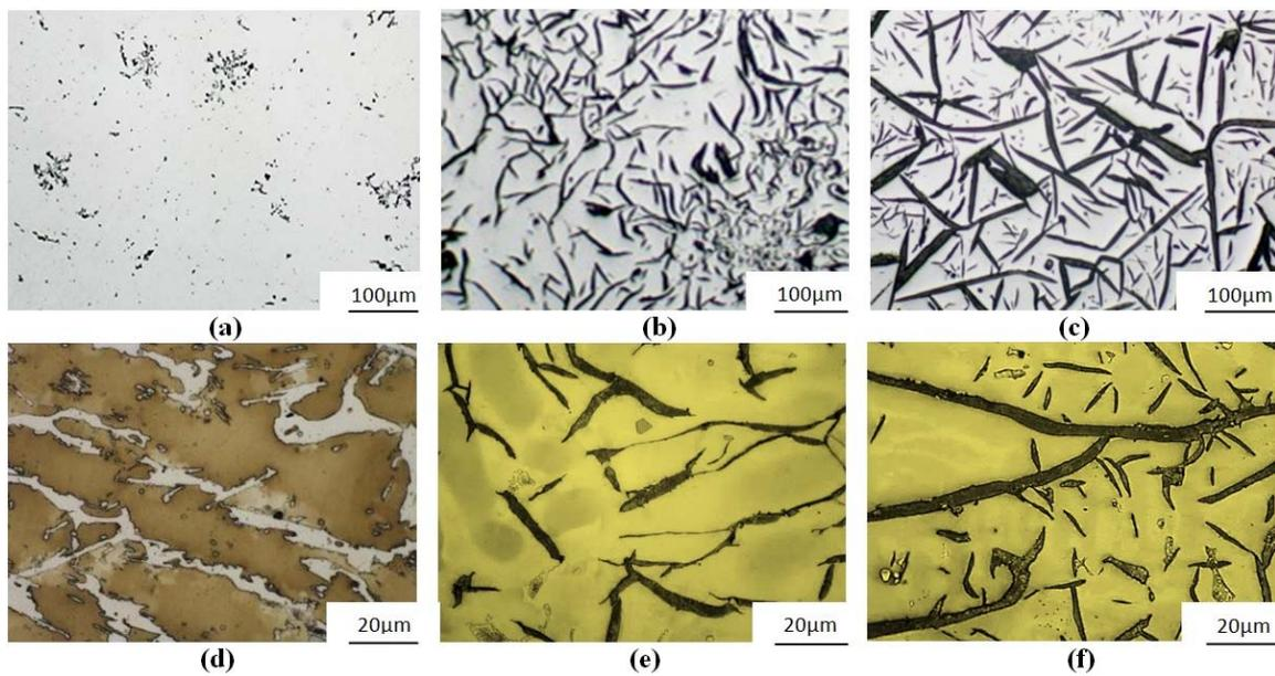
**Figure 1.** Austenitic cast iron Ni-Mn-Cu: (a) No. 1—trace amounts of nodular graphite ID8; (b) No. 2—flake straight graphite (IA4) with some features indicating type B arrangement; (c) No. 3—primary graphite IC3; (d) No. 1—subeutectic, chilled structure ( $Equ_{Ni} = 19.4\%$ ,  $S_C = 0.55$ ); (e) No. 2—eutectic with flake graphite ( $Equ_{Ni} = 18.7\%$ ,  $S_C = 1.06$ ); (f) No. 3—hypereutectic ( $Equ_{Ni} = 17.1\%$ ,  $S_C = 1.48$ ); (a–c) unetched; (c–e) etched with Mi1Fe.
