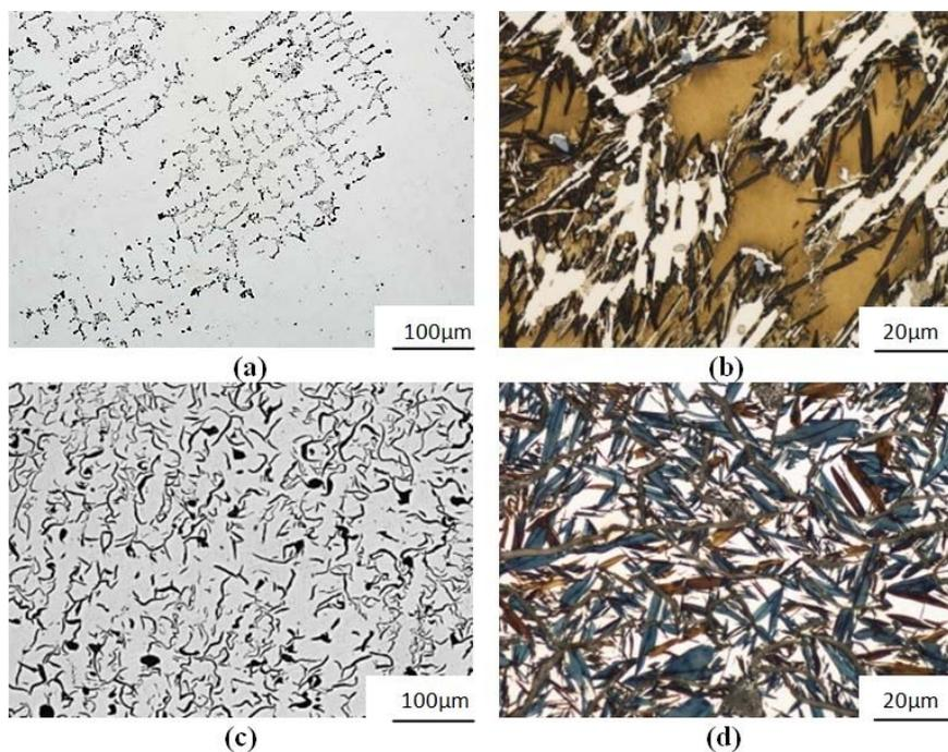
**Figure 2.** Cast iron Ni-Mn-Cu: (a) No. 4—subeutectic with a small number of interdendritically arranged colonies of ID7 graphite; (b) No. 4—chilled after partial austenite-martensite transition ( $Equ_{Ni} = 13.6\%$ ,  $S_C = 0.66$ ); (c) No. 5—graphite colonies characteristic for eutectic alloy IA5 with graphite features indicating interdendritic arrangement type E; (d) No. 5—martensite after the transformation ( $Equ_{Ni} = 11.6\%$ ,  $S_C = 0.98$ ). (a,c) unetched; (b,d) etched with Mi1Fe.
