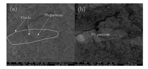
Figure 9. Fracture surface of tensile specimen tested at room temperature: (a) shows the region initiating the fracture in the secondary-electron emission model; (b) shows the BSE fracture corresponding to (a).
