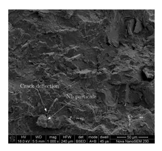
**Figure 11.** The fracture surface of the 3PB Ti-45Al-5Nb-0.4W/2Nb (at. %) alloy with a DP microstructure tested at room temperature with a loading rate of 0.05 mm/min.
