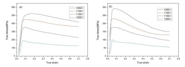
**Figure 3.** Flow curves of the Ti-45Al-5Nb-0.4W/2Nb (at. %) alloy at: (a)  $1 \text{ s}^{-1}$  and different temperatures; (b)  $0.01 \text{ s}^{-1}$  and different temperatures.
