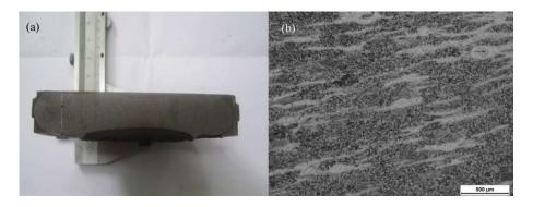
**Figure 8.** Hot pack forging of a Ti-45Al-5Nb-0.4W/2Nb (at. %) alloy billet: (a) the cross-section of the deformed billet; (b) the optical metallographic microstructure in the center of the billet after heat treatment of  $1260 \,^{\circ}\text{C/2}$  h with air cooling.
