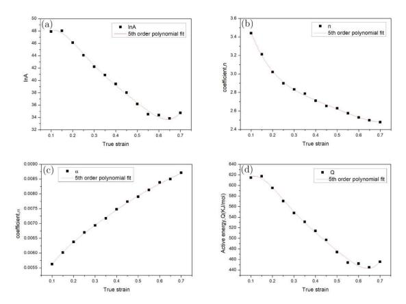
**Figure 4.** Plots used for calculation of: (a) A, (b) n, (c)  $\alpha$ , and (d) deformation activation energy.
