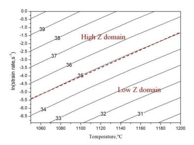
**Figure 5.** Zener-Hollomon parameter ( $\ln Z$ ) of the Ti-45Al-5Nb-0.4W/2Nb (at. %) alloy at different temperatures and strain rates (the numbers on the contour lines are the values of  $\ln Z$ ).
