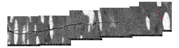
**Figure 10.** Crack path of the Ti-45Al-5Nb-0.4W/2Nb (at. %) alloy with a DP microstructure tested at room temperature with a loading rate of 0.05 mm/min.
