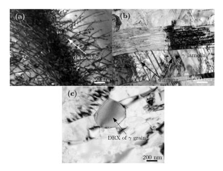
**Figure 7.** TEM images of Ti-45Al-5Nb-0.4W/2Nb (at. %) deformed to a true strain of 0.7 at different Z values: (**a**,**b**)  $\ln Z = 40.44$  (high Z,  $1050 \,^{\circ}\text{C}/1 \, \text{s}^{-1}$ ); (**a**) shows the high density of dislocations in  $\gamma$  grains; (**b**) shows the residual lamellar colony with the dislocations and twins; (**c**) shows the recrystallized  $\gamma$  grain at  $\ln Z = 30.70$  (low Z,  $1150 \,^{\circ}\text{C}/0.001 \, \text{s}^{-1}$ ).
