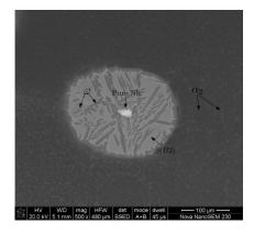
Figure 2. Microstructure of the Ti-45Al-5Nb-0.4W/2Nb (at. %) alloy before compression.
