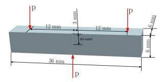
Figure 1. Shapes and dimensions of bending specimen (mm).
