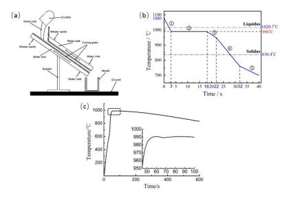
**Figure 2.** Schematic illustration of the: (a) ECSC equipment; (b) forming process curve; and (c) temperature recording curve during slurry transfer ① ECSC process, ② slurry transfer, ③ mold filling, ④ holding pressure, ⑤ parts air cooling.
