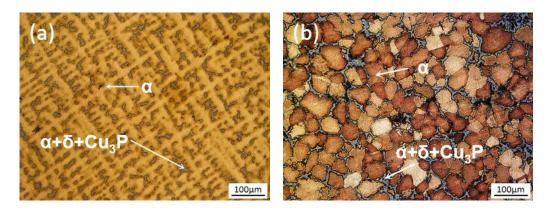
Figure 4. Microstructures of ZCuSn10P1 alloy: (a) as-cast; and (b) semi-solid.
