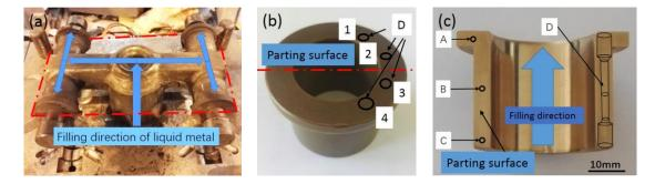
**Figure 3.** Mold map and the product of ZCuSn10P1 alloy: (**a**) mold map; and (**b**,**c**) squeeze part (A, B and C are sampling positions for microstructure observation, while D is sampling position and shape for tensile test, 1 to 4 are sampling positions for tensile test from above the parting surface to below the parting surface).
