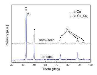
Figure 5. XRD spectrum of ZCuSn10P1 alloy.
