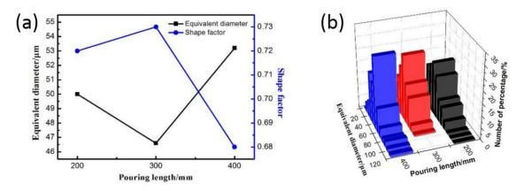
**Figure 8.** Relationship between equivalent diameter and shape factor of primary  $\alpha$ -Cu phase with pouring length (**a**); and distribution of primary  $\alpha$ -Cu phase equivalent diameter (**b**) at different pouring lengths of semi-solid ZCuSn10P1 alloy.
