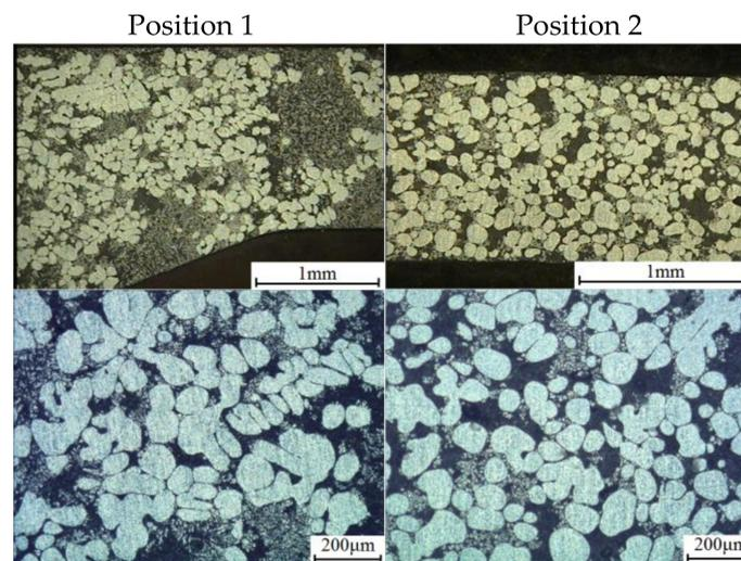
**Figure 9.** Microstructure of a thin plate fabricated using 60 A stirred 45%-solid-fraction billet, graphite lubricant, 200 MPa of pressure, and 30 mm/s velocity.
