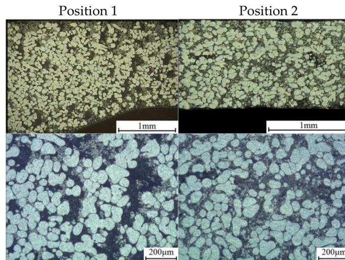
**Figure 8.** Microstructure of a thin plate fabricated using 60 A stirred 45%-solid-fraction billet, graphite lubricant, 100 MPa of pressure, and 300 mm/s velocity.
