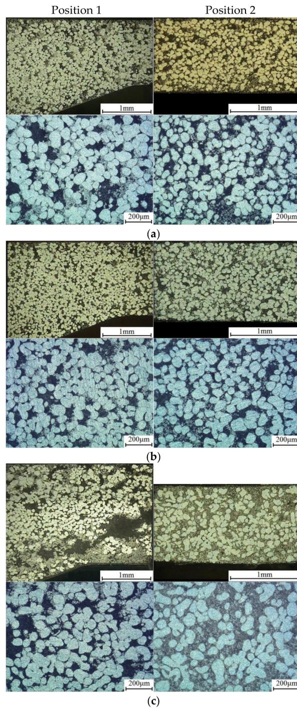
**Figure 7.** Microstructure of thin plates fabricated using 60 A stirred billets (graphite lubricant, 200 MPa of pressure and 300 mm/s of velocity): (a) Using a billet with 35% solid fraction; (b) Using a billet with 45% solid fraction; (c) Using a billet with 55% solid fraction.
