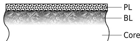
**Figure 1.** Schematic cross-section of alloy architecture before low-temperature carburization. (Core: alloy core with bulk properties. BL: Beilby layer. PL: Passivating Cr-rich oxide layer.
