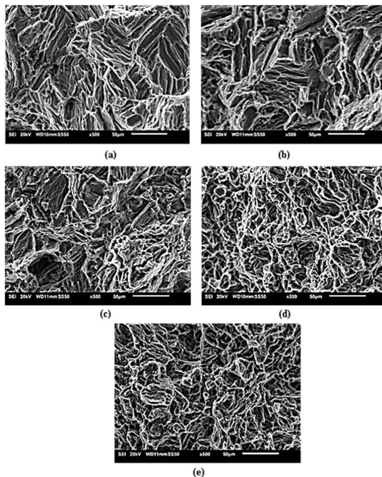
**Figure 5.** Tensile fractography of (a) Pure Mg, (b) Mg0.5NiTi, (c) Mg1NiTi, (d) Mg1.5NiTi and (e) Mg3NiTi nanocomposites.
