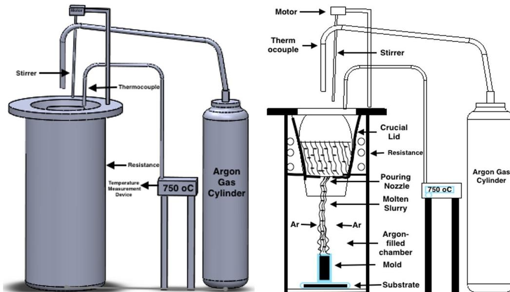
Figure 1. Experimental setup of the DMD method.
