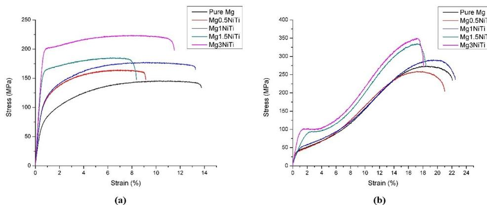
**Figure 4.** (a) Tensile and (b) compressive stress vs. strain curve obtained for different Mg-NiTi nanocomposites.
