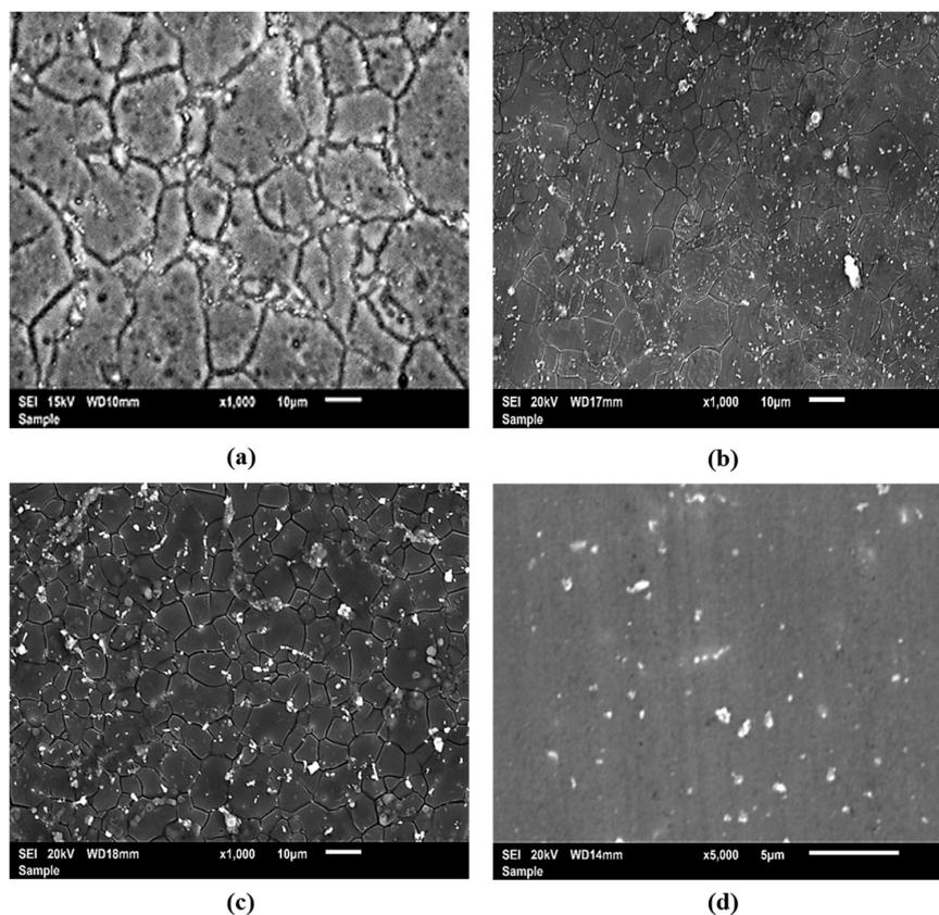
**Figure 2.** Grain size of (a) pure Mg, (b) Mg1.5NiTi, (c) Mg3NiTi; (d) NiTi distribution in the Mg matrix.
