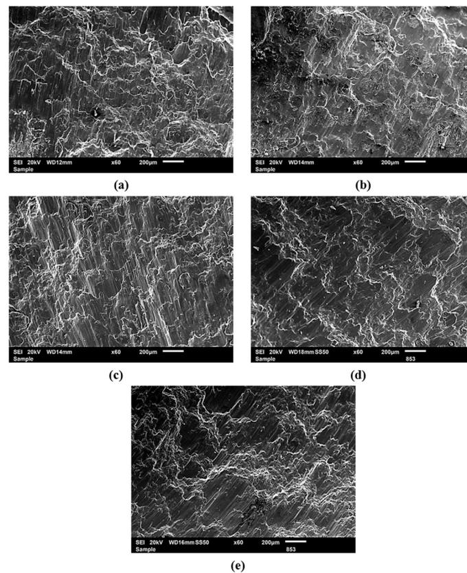
**Figure 6.** Compression fractography of (a) Pure Mg, (b) Mg0.5NiTi, (c) Mg1NiTi, (d) Mg1.5NiTi and (e) Mg3NiTi nanocomposites.
