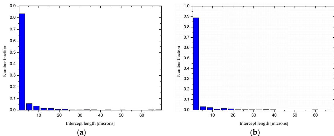
**Figure 7.** Grain size distribution of the AlMg5 alloy samples (a) ST + ECAP 2× + ageing 160 °C for 4 h and (b) ST + ECAP 2× + ageing 180 °C for 4 h.
