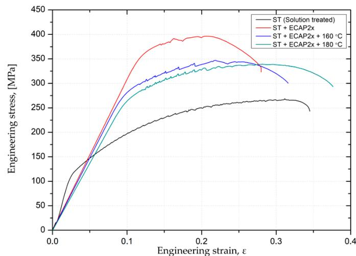
**Figure 9.** Comparison of engineering stress-engineering strain curves for the AlMg5 alloy subjected to different types of treatments.
