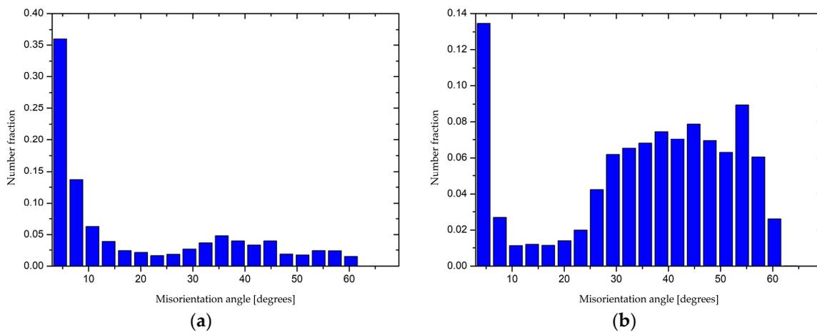
**Figure 6.** Misorientation angle distribution of the AlMg5 alloy samples (a) ST + ECAP 2× + ageing 160 °C for 4 h and (b) ST + ECAP 2× + ageing 180 °C for 4 h.
