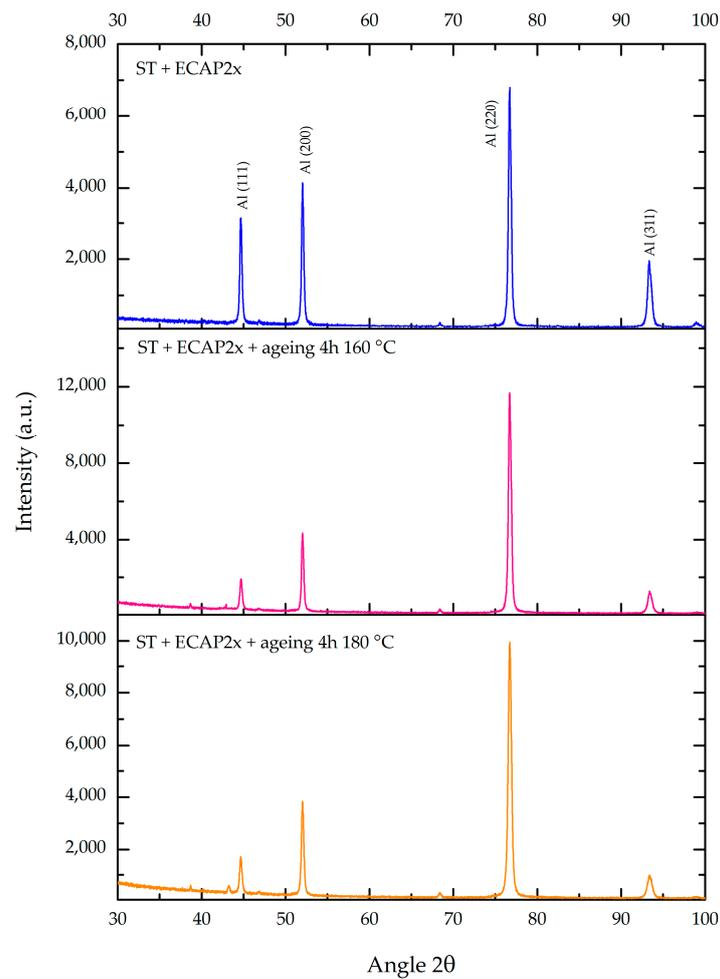
**Figure 8.** X-ray diffraction pattern of the AlMg5 specimens.
