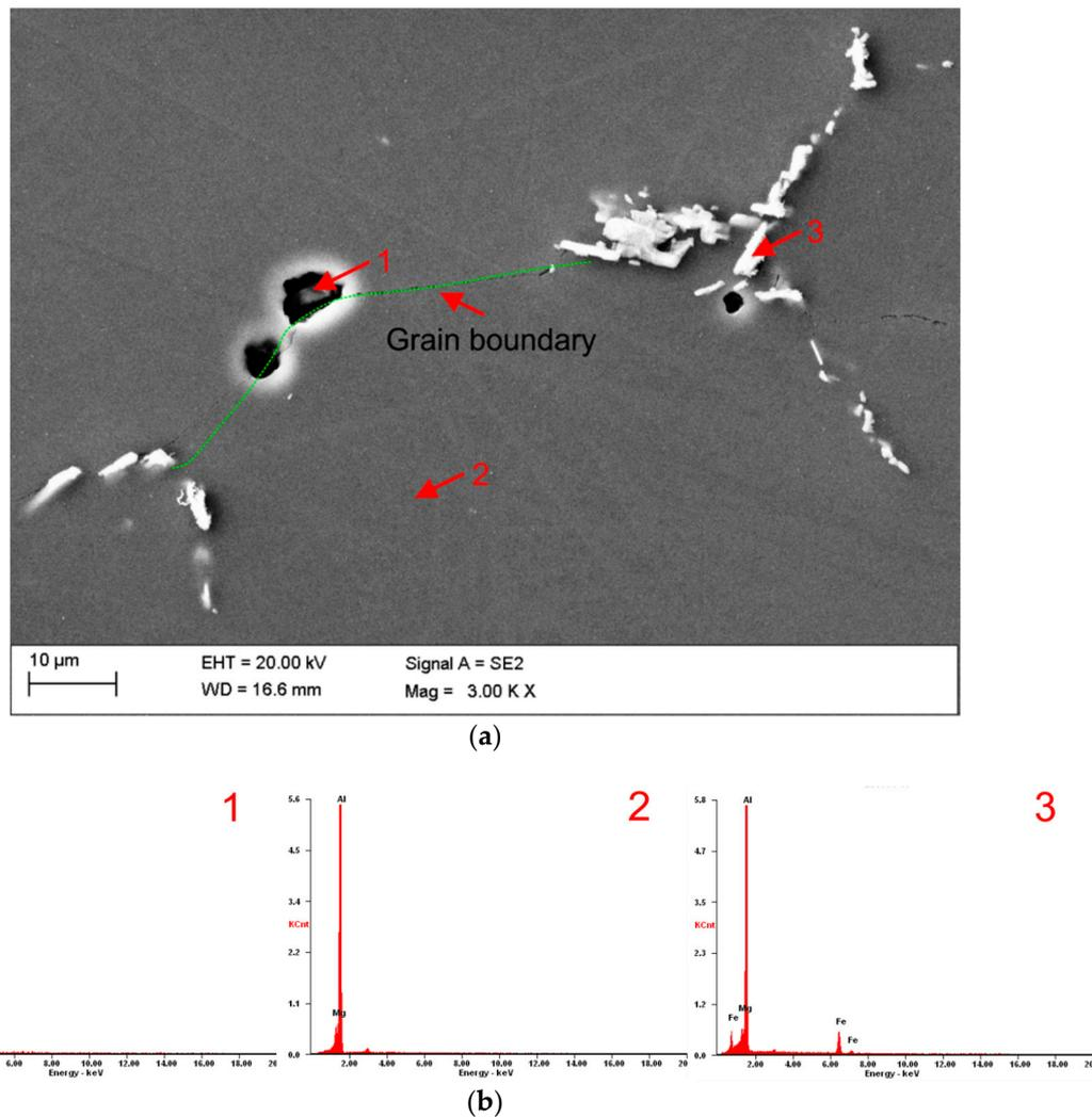
**Figure 2.** Secondary electron image of a solution-treated AlMg5 alloy (a) and corresponding EDS spectra of the analysed phases (b).
