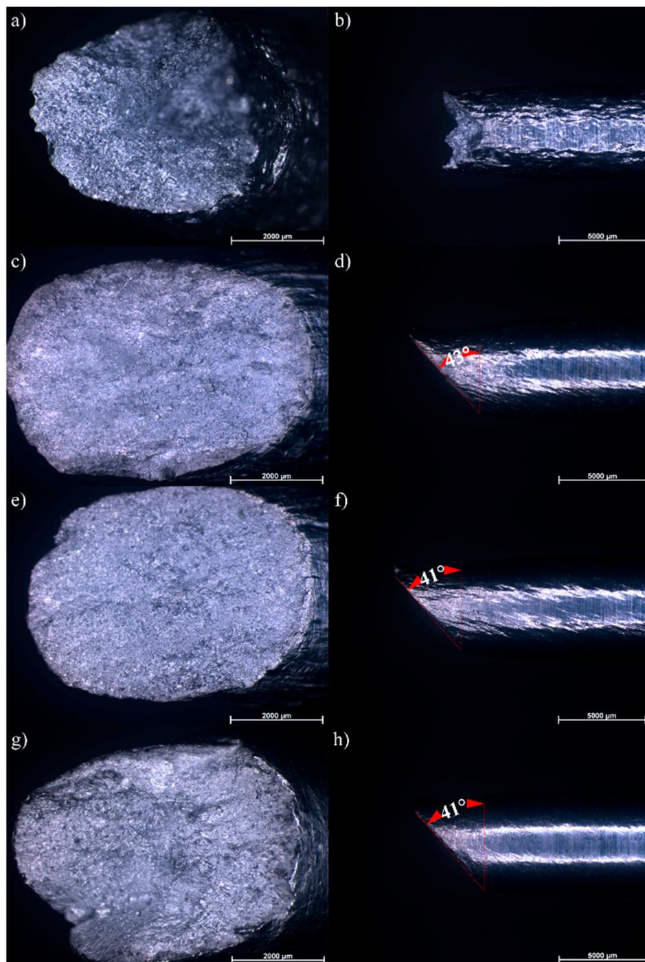
**Figure 10.** Fracture surfaces of as-built vertical and horizontal samples: (a) and (b) solution-treated (ST); (c) and (d) ST + ECAP 2 $\times$ ; (e) and (f) ST + ECAP 2 $\times$  + ageing  $160^\circ\text{C}$  for 4 h; and (g) and (h) ST + ECAP 2 $\times$  + ageing  $180^\circ\text{C}$  for 4 h.
