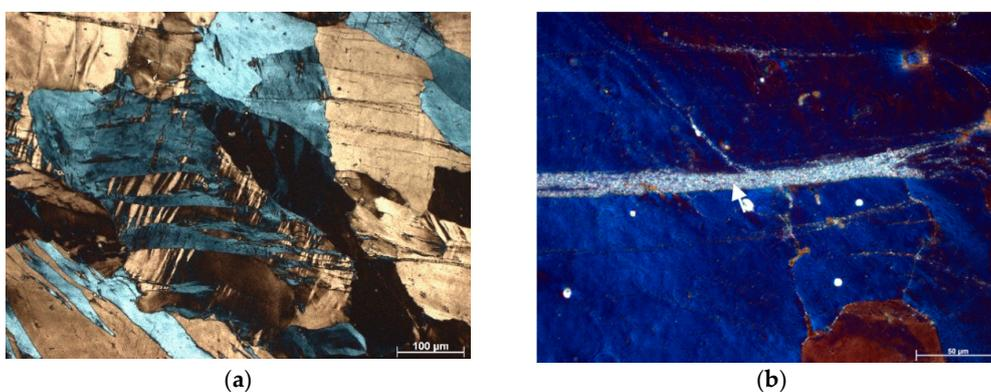
**Figure 4.** Microstructures of the AlMg5 samples (a) ST + ECAP 2 $\times$  + ageing 160 °C for 4 h, (b) ST + ECAP 2 $\times$  + ageing 180 °C for 4 h.
