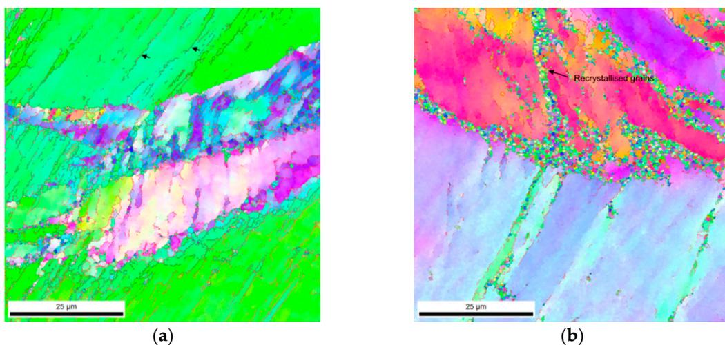
**Figure 5.** Electron backscatter diffraction (EBSD) IPF (Inverse Pole Figure) maps achieved from the centre region of the specimens (cross-section view) (a) ST + ECAP  $2\times$  + ageing  $160^\circ\text{C}$  for 4 h and (b) ST + ECAP  $2\times$  + ageing  $180^\circ\text{C}$  for 4 h.
