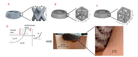
**Figure 1.** Designs of artificial acetabular cups with an open-porous load-bearing unit cell in a reduced variant; (**A**) Illustration—twisted unit cell, (**B**) Illustration—combined unit cell, (**C**) Illustration—combined open unit cell substitute, (**D**) Press-fit area and gap in case of reduced cup model (negative press-fit)—schematic figure and photograph, all units are in mm.
