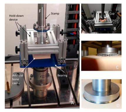
**Figure 3.** Pull-out-test setup—(**A**) Complete experimental setup; (**B**) Cup ready for pressing in; (**C**) View from upside of the acetabular cup with artificial bone cavity and the pull-out stamp; (**D**) Cup completely press-fitted.
