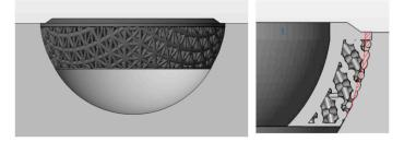
**Figure 2.** The cup is positioned in the artificial bone cavity (**left**) and the area virtually penetrates the artificial bone cavity-red hatched area (**right**). This area describes the Press-fit volume.
