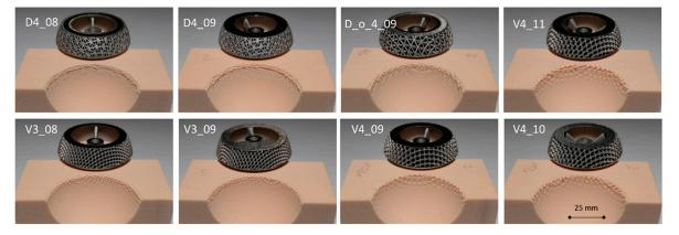
**Figure 11.** Representative imaging of mechanical deformations in the artificial bone cavity for cup design usage in lever-out test.
