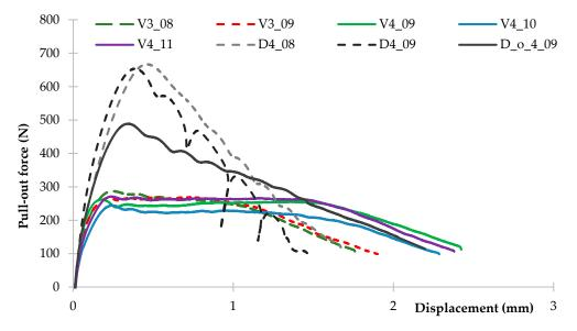
Figure 6. Representative force-displacement curve of the pull-out tests for each cup design.
