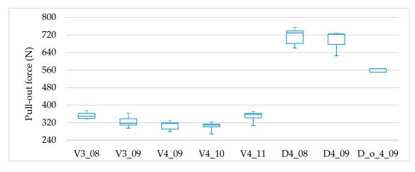
**Figure 5.** Boxplots of the measured pull-out force (N). Boxplots indicate the median value, the interquartile range (IQR: interval between the 25th and 75th percentile, blue rectangle) and the extremum values (n = 5).
