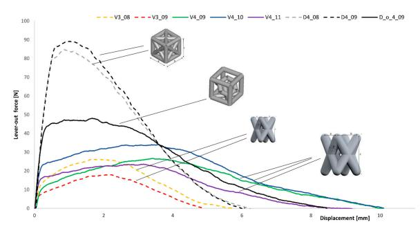
Figure 10. Representative lever-out force vs. displacement curve of the lever-out test for each cup design.
