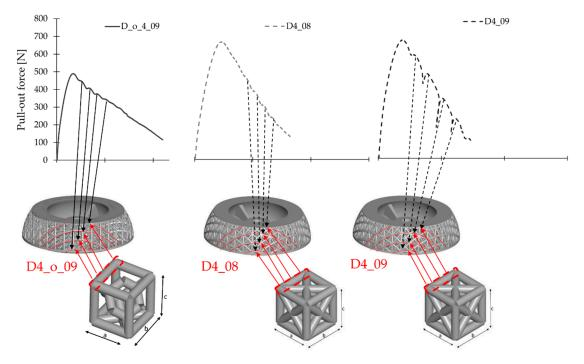
Figure 7. Representation of the cascades with reference to the structure on the cup surface.
