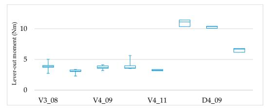
**Figure 9.** Boxplots of the measured lever-out moments (Nm). Boxplots indicate the median value, the interquartile range (IQR: interval between the 25th and 75th percentile, blue rectangle) and the extremum values (n = 5).
