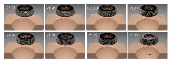
Figure 8. Representative pictures of the bone cavities after the pull-out test for each cup design.
