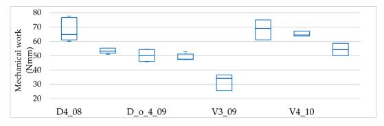
**Figure 12.** Boxplots of the measured mechanical work (Nmm) during the lever-out test. Boxplots indicate the median value, the interquartile range (IQR: interval between the 25th and 75th percentile, blue rectangle) and the extremum values (n = 5).
