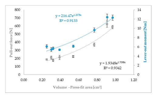
**Figure 13.** Pull-out force as calculated from pull-out testing and volume press-fit area as well as lever-out moment as calculated from lever-out testing for the eight cup-designs. Results are shown as mean values with the corresponding standard deviation (n = 5 for each design).
