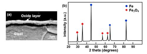
**Figure 3.** (a) Cross-sectional SEM image of the surface of steel hot-dipped in liquid Al at 690 °C for 30 s and (b) XRD analysis of the surface. The oxide layer formed on the steel surface.
