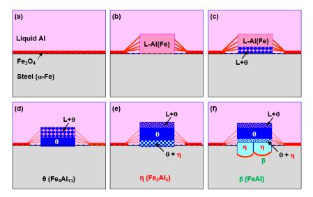
**Figure 11.** Schematic diagram of the nucleation process of the reaction layer and phases during the hot-dipping of steel in liquid Al at 690°C. (a) Initial stage of hot-dipping; (b) Oxide film breaks and dissolution-diffusion of Fe; (c) nucleation of  $\theta$  phase; (d) growth of  $\theta$  phase; (e) nucleation of  $\eta$  phase; (f) growth of  $\eta$  phase and generation of  $\beta$  (FeAl) phase.
