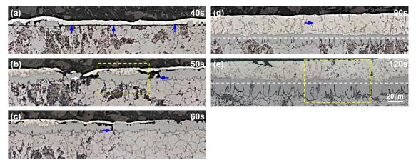
**Figure 7.** Cross-sectional optical micrograph of specimens hot-dipped at 690 °C for (**a**) 40 s, (**b**) 50 s, (**c**) 60 s, (**d**) 90 s, and (**e**) 120 s.
