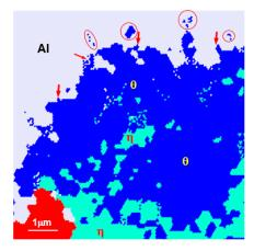
**Figure 13.** Enlarged view of the EBSD phase map in Figure 6a. Al and  $\theta$  phase region observed on the left side.
