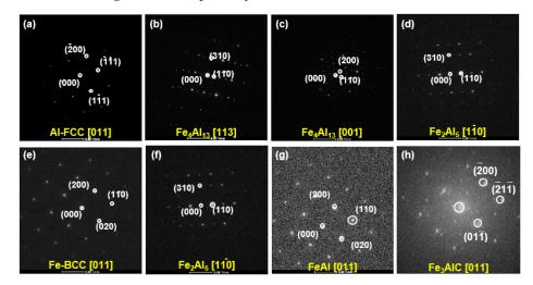
**Figure 5.** (**a**–**h**) Diffraction patterns and the selected diffraction pattern for the areas marked 1–8 in Figure 4, respectively.
