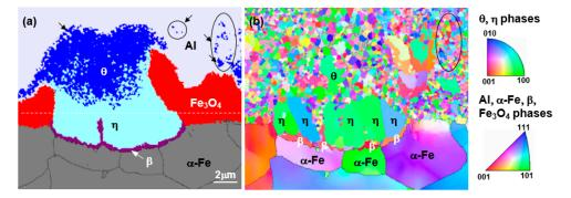
**Figure 6.** (a) Electron backscatter diffraction (EBSD) phase map and (b) Inversed Pole Figure (IPF) of the specimen hot-dipped in pure Al melt at 690 °C for 30 s in Figure 2.
