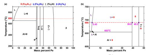
**Figure 12.** Fe-Al binary phase diagram calculated using ThermoCalc<sup>TM</sup> software ver 6.0 (Solna, Sweden). (**a**) Fe: 0–100%; (**b**) Fe: 0–50%.
