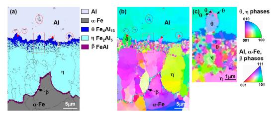
**Figure 10.** (**a**) EBSD phase map (**b**) IPF, and (**c**) magnified view for the rectangular area of specimen hot-dipped in liquid Al melt for 120 s.
