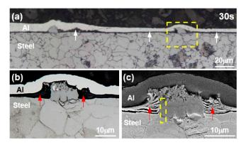
**Figure 1.** (**a**) Optical microscopy of hot-dipped specimen reaction layer in liquid Al melt at 690  $^{\circ}$ C for 30 s, (**b**) magnified view, and (**c**) SEM image of the dotted rectangular area in (**a**).
