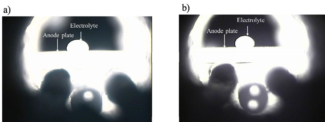
**Figure 10.** Wetting angles of electrolyte on anodes at 1215 K. (a) the carbon anode; (b) the graphite anode.
