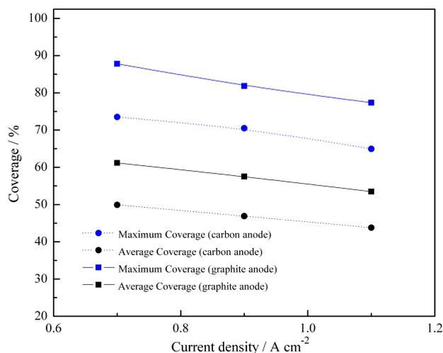
**Figure 9.** Gas coverage as a function of anodic current density for the carbon and graphite anodes.
