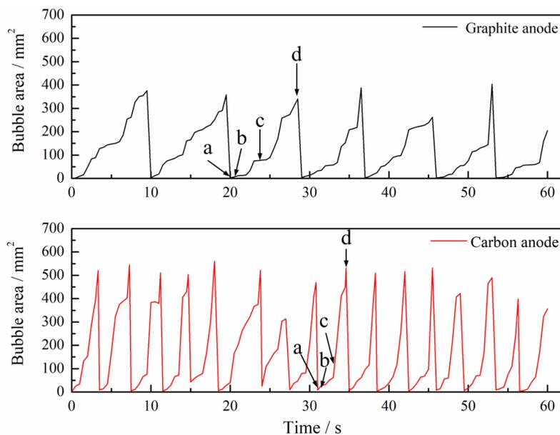
**Figure 7.** Fluctuation in the largest bubble area on the carbon and graphite anodes over time. a-stage 1; b-stage 2; c-stage 3; d-stage 4.
