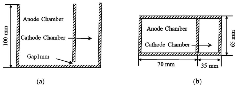
**Figure 2.** Double-chamber quartz crucible showing the anode and cathode chamber. (a) front view; (b) top view.
