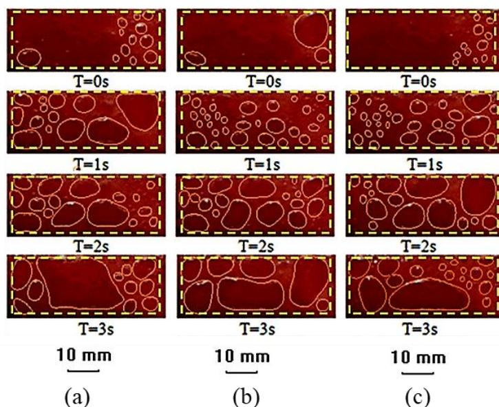
**Figure 11.** Bubble generation-growth-releasing process on the carbon anode. (a) the 1st period; (b) the 2nd period; (c) the 3rd period.
