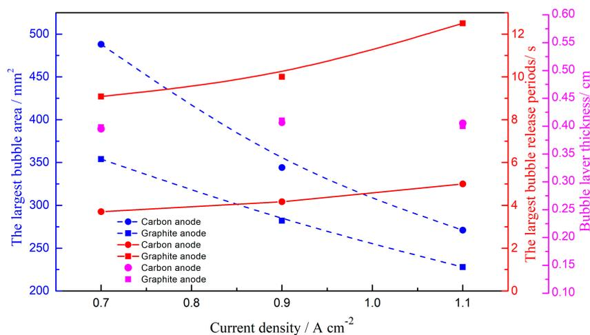
**Figure 8.** The largest bubble area, the release periods and bubble thickness as a function of anodic current density for the carbon and graphite anodes.
