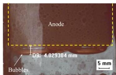
**Figure 4.** Measurement for the thickness of the bubble layer from side observations.
