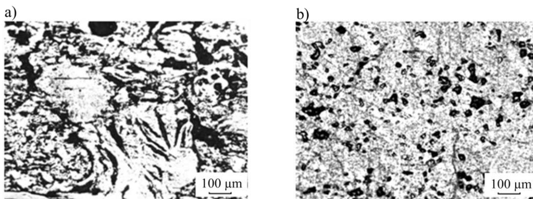
**Figure 6.** Optical microscopy images of the (a) carbon and (b) graphite anodes.
