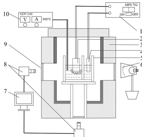
**Figure 1.** Schematic diagrams of the transparent electrolysis cell. 1: DC power supply; 2: anode; 3: furnace; 4: cathode; 5: quartz crucible; 6: light source; 7: computer; 8: industrial cameras; 9: quartz window; 10: CKW-3100 temperature controller.
