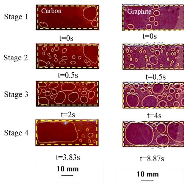
**Figure 5.** Comparison of bubble behavior between carbon and graphite anodes at a current density of  $0.7 \text{ A}\cdot\text{cm}^{-2}$ . Stage 1: Just after bubble release; Stage 2: Bubble growth; Stage 3: Bubble growth and coalescence; stage 4: Just before bubble release.
