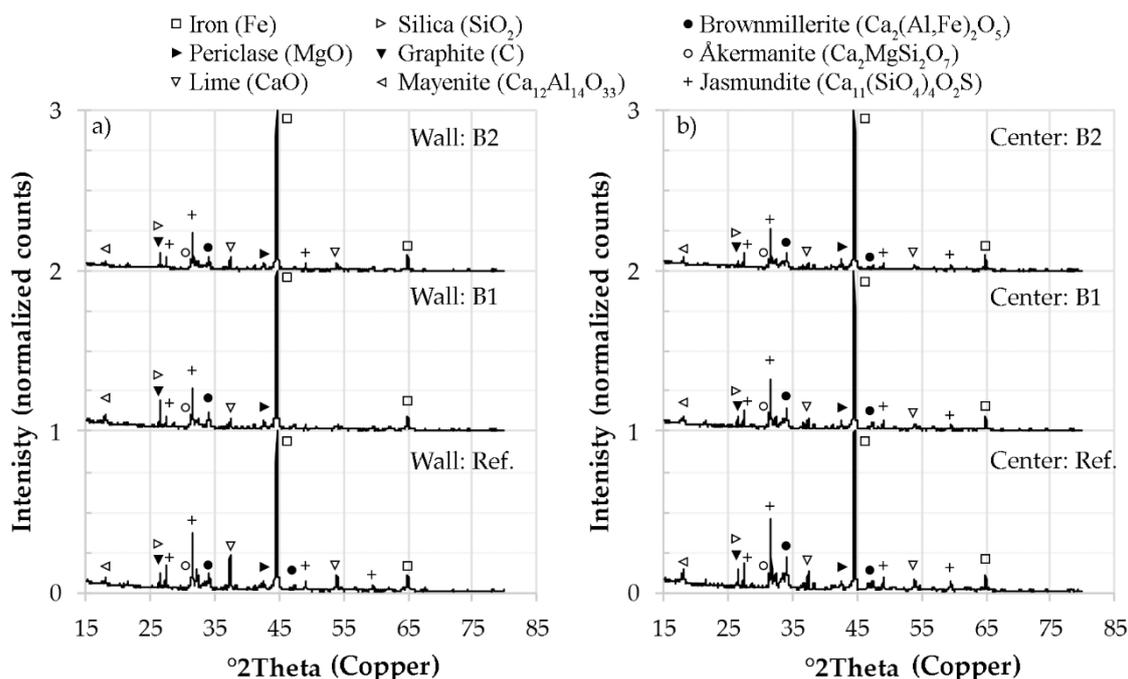
**Figure 4.** Diffractograms of the briquettes that have gone through the (a) wall program and (b) center program of the laboratory-scale BF experiments.
