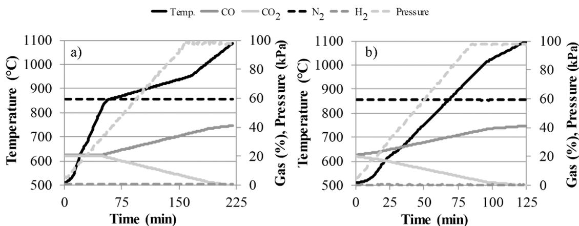
**Figure 2.** Heating profile, gas profile, and mechanical pressure during the (a) wall program and (b) center program of the laboratory-scale BF experiment.
