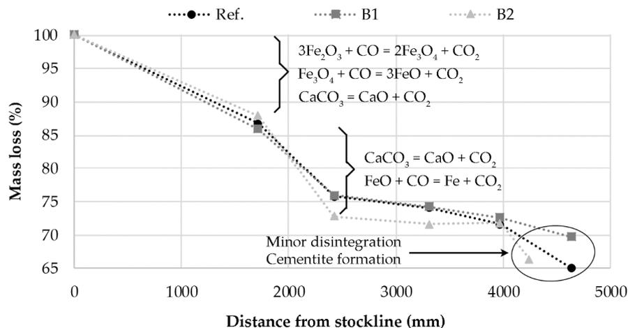
**Figure 5.** Mass loss and reactions during the descent of the briquettes in the LKAB EBF.
