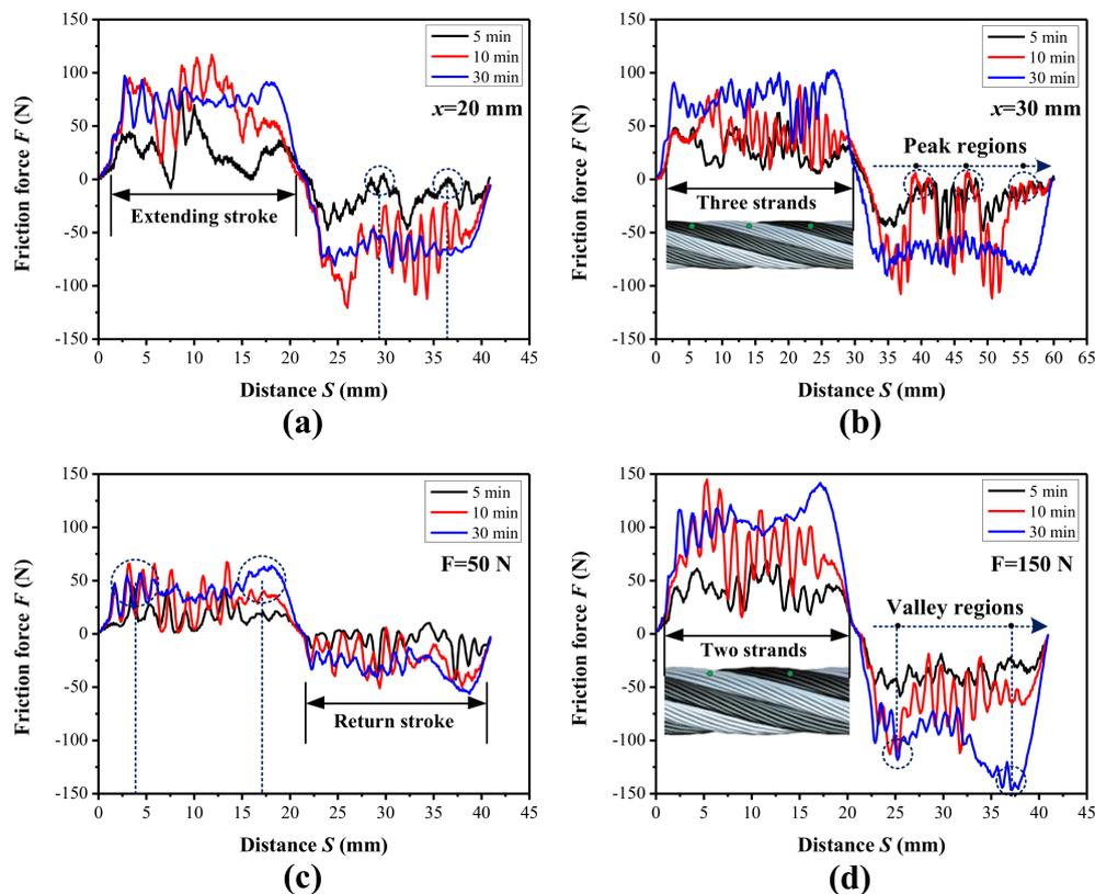
**Figure 3.** The evolution of friction force over one cycle for different periods. (a) Stroke: 20 mm, load: 100 N; (b) stroke: 30 mm, load: 100 N; (c) load: 50 N, stroke 20 mm; (d) load: 150 N, stroke: 20 mm.
