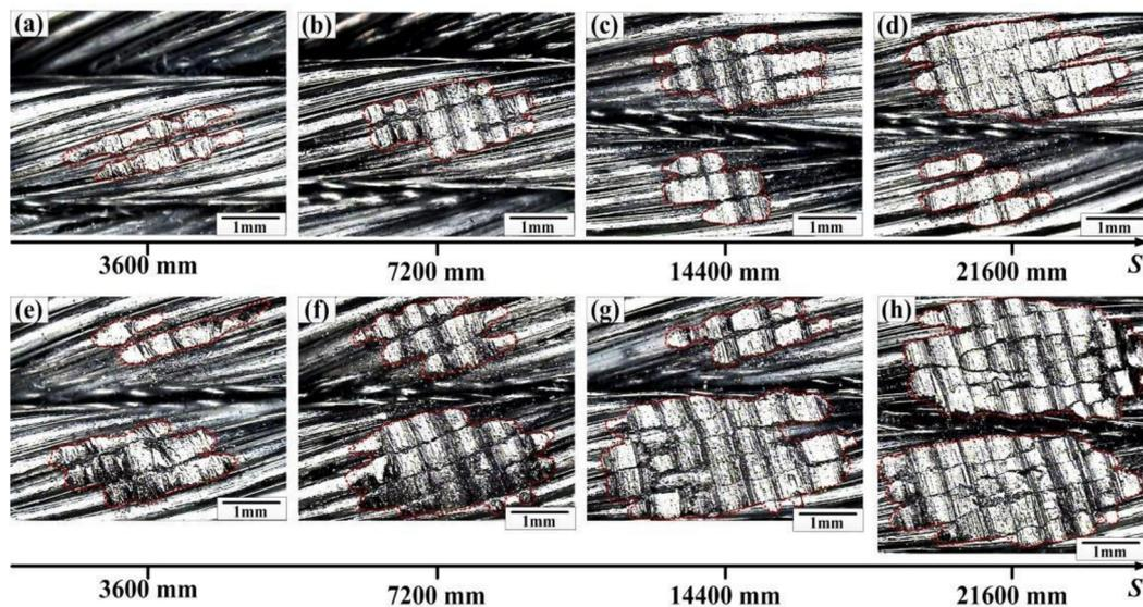
**Figure 10.** Optical micrographs of the wear scars under different loads. (a–d) Load: 50 N, stroke: 20 mm; (e–h) load: 150 N, stroke: 20 mm.
