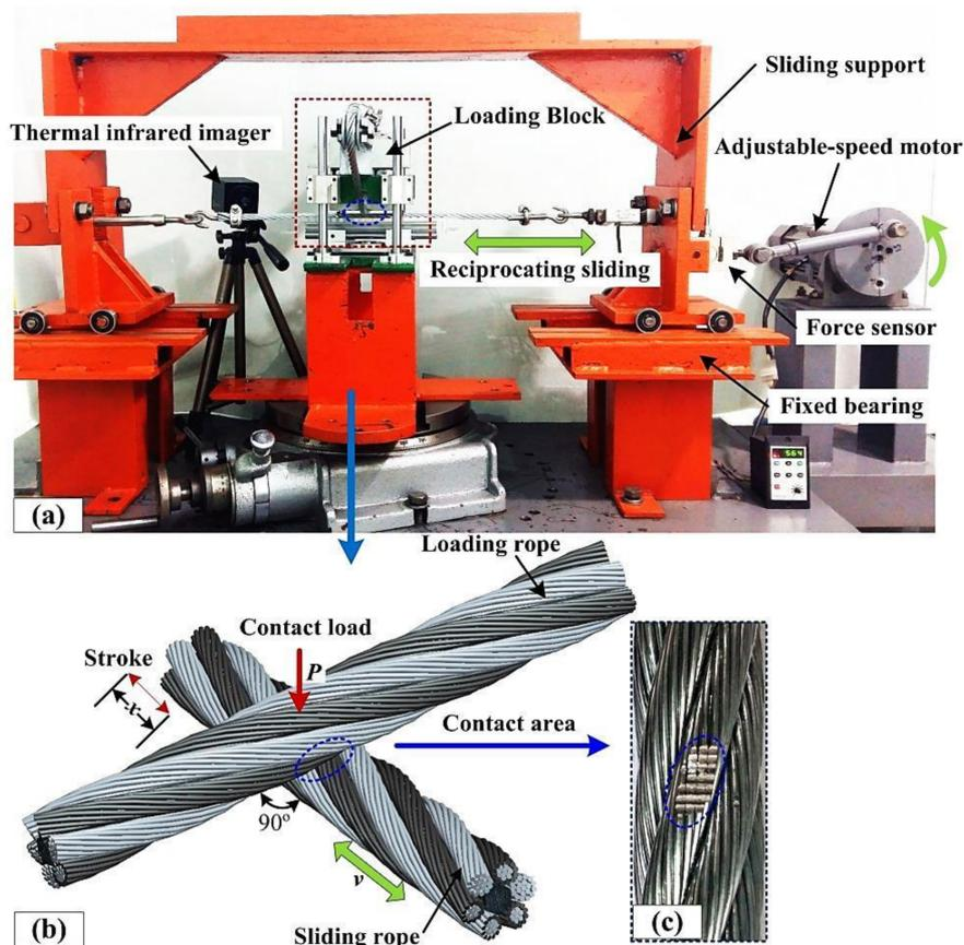
Figure 2. Sliding friction test rig of wire rope. (a) Test rig; (b) contact form; (c) wear scar.
