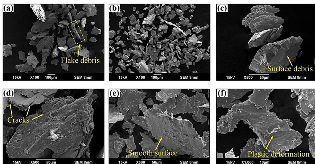
**Figure 11.** Scanning electron microscopy (SEM) micrographs of the wear debris with different magnifications. (a,d)  $\times 100$ ; (c–e)  $\times 500$ ; (f)  $\times 1000$ .
