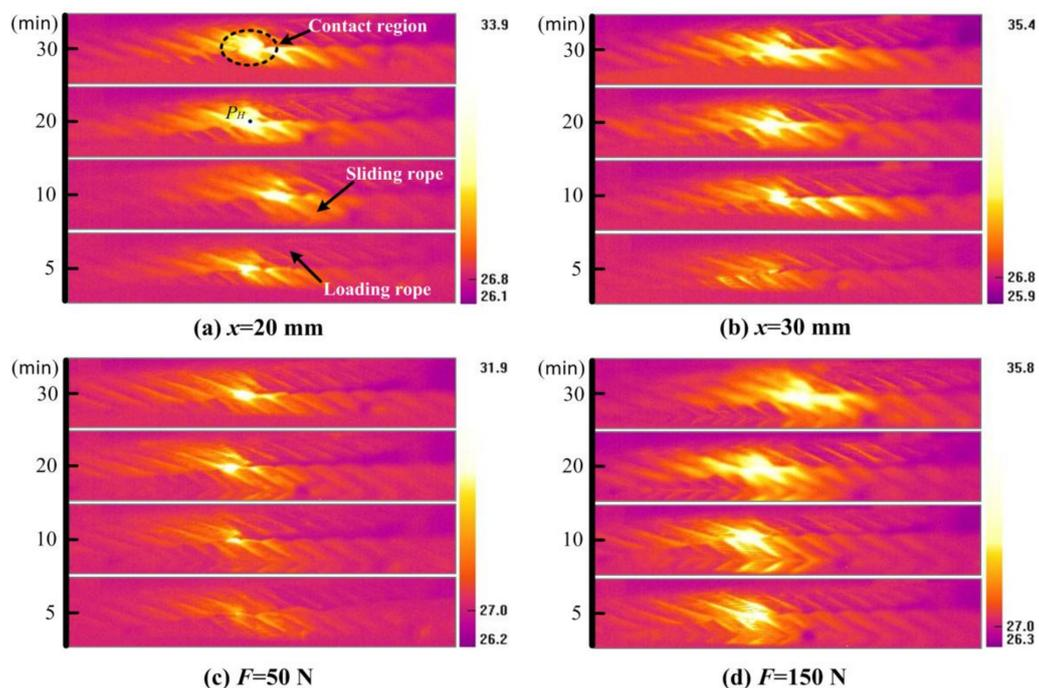
**Figure 6.** Infrared thermograms of contact wire ropes at different stages. (a) Stroke: 20 mm, load: 100 N; (b) stroke: 30 mm, load: 100 N; (c) load: 50 N, stroke: 20 mm; (d) load: 150 N, stroke: 20 mm.
