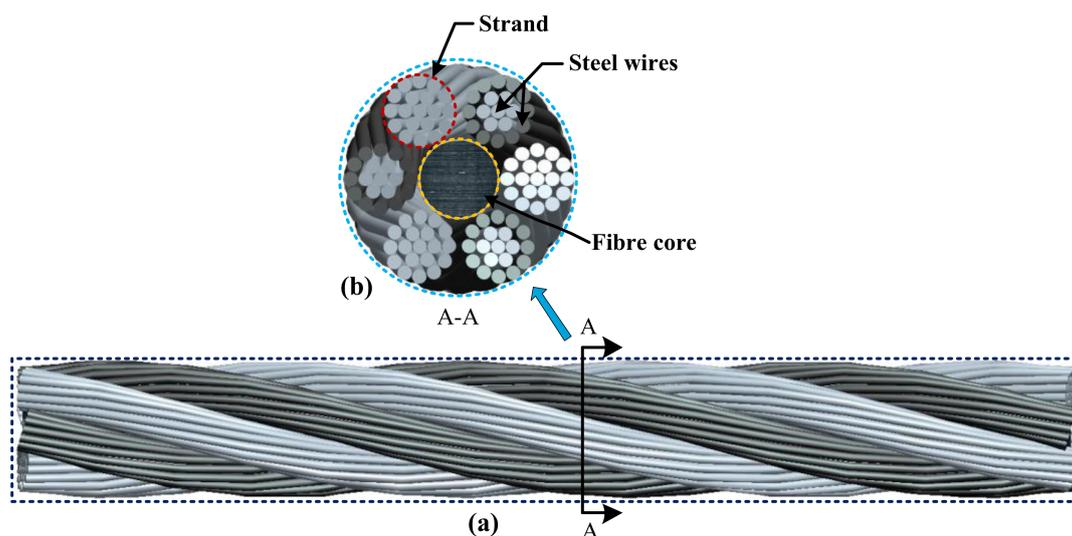
**Figure 1.**  $6 \times 19 + FC$  wire rope sample. (a) wire rope; (b) cross section.
