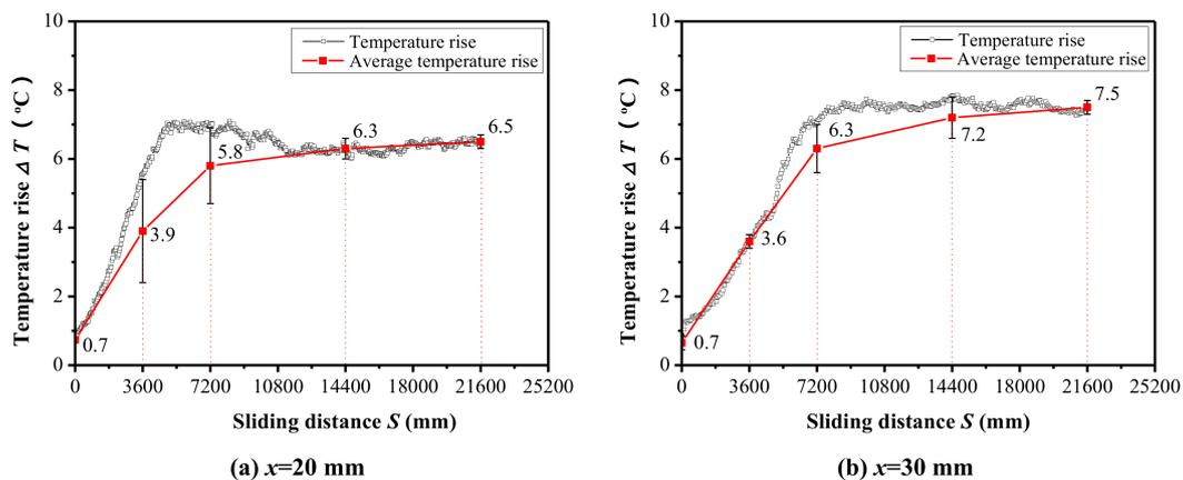
**Figure 7.** The evolution of temperature rise under different strokes. (a) Stroke: 20 mm, load: 100 N; (b) stroke: 30 mm, load: 100 N.
