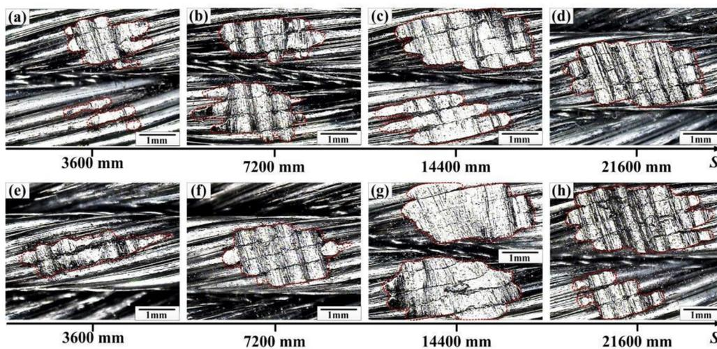
**Figure 9.** Optical micrographs of the wear scars under different strokes. (a–d) Stroke: 20 mm, load: 100 N; (e–h) stroke: 30 mm, load: 100 N.
