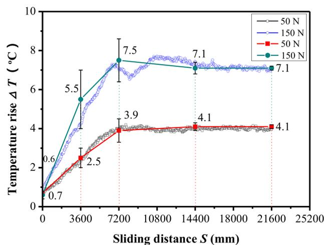
**Figure 8.** The evolution of temperature rise under different contact loads ( $x$ : 20 mm).
