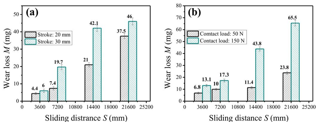
**Figure 12.** The evolution of wear mass loss for the wire rope under different conditions. (a) Stroke: 20 mm and 30 mm, load: 100 N; (b) load: 100 N and 150 N, stroke: 20 mm.
