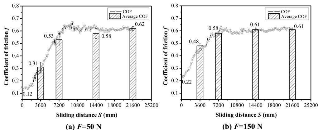
**Figure 5.** The evolution of the coefficient of friction under different contact loads. (a) Load: 50 N, stroke: 20 mm; (b) load: 150 N, stroke: 20 mm.
