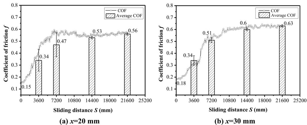
**Figure 4.** The evolution of the coefficient of friction under different strokes. (a) Stroke: 20 mm, load: 100 N; (b) stroke: 30 mm, load: 100 N.
