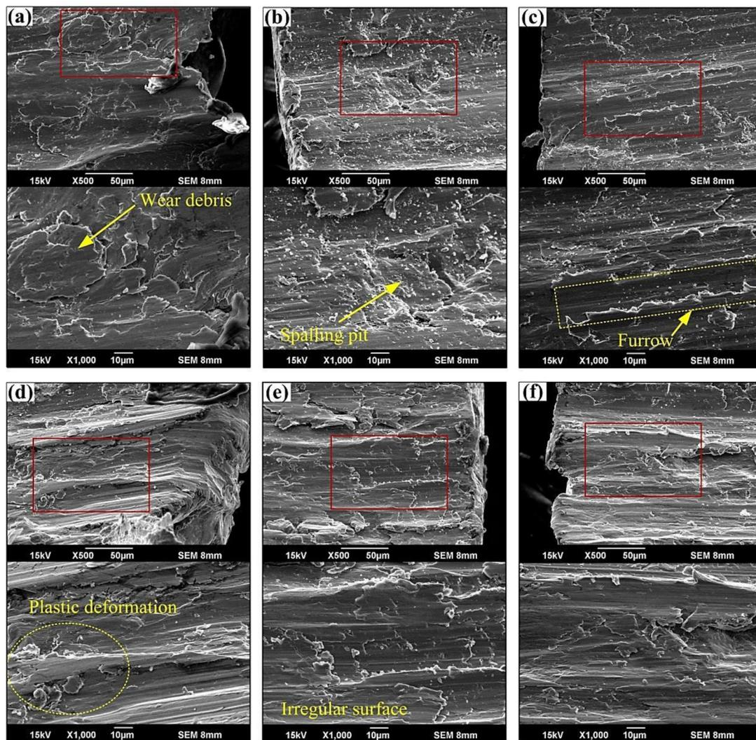
**Figure 13.** SEM micrographs of the wear surfaces with different morphology properties. (a–c) Relatively regular surface; (d–f) irregular surface.
