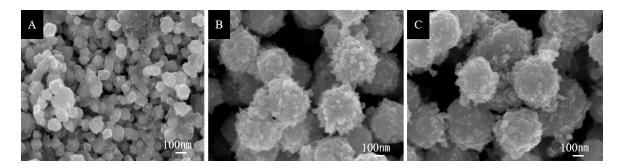
**Figure 1.** Field emission scanning electron microscopy (FE-SEM) images of reduced nickel particle: **(A)** NaOH of 10 g; **(B)** NaOH of 12.5 g; **(C)** NaOH of 15 g.
