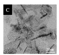
**Figure 2.** Field emission transmission electron microscopy (FE-TEM) images of synthesized nickel particle: **(A)** no addition of PVP; **(B)** PVP of 1 g; **(C)** PVP of 2 g.
