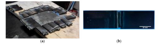
**Figure 3.** Test specimens after Nickel filler metal deposition: (**a**) welded Nickel bead to chamfer edge; and (**b**) re-chamfered edges after Nickel deposition.
