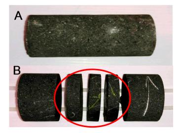
**Figure 3.** Anode core shapes for measuring electrical resistivity using the standard method (**A**) and the Van der Pauw method (**B**).
