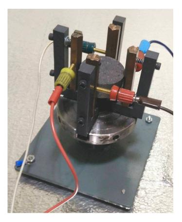
**Figure 2.** Picture of the Van der Pauw setting for laboratory measurement. The sample is placed at the center, between the four V-shaped copper probes.
