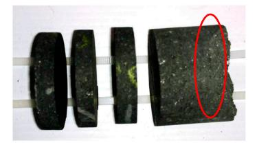
**Figure 4.** Broken sample prepared for measurement using the Van der Pauw method. The failure was circled at the right of the sample.
