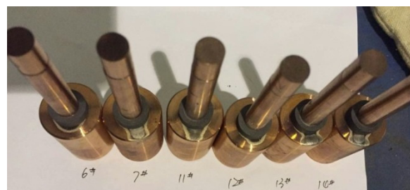
Figure 15. The brazed samples with side solder feeding.
