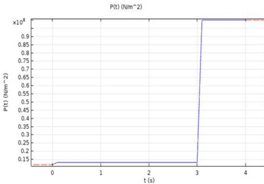
**Figure 10.** Pressure applied for the welding of similar metals.
