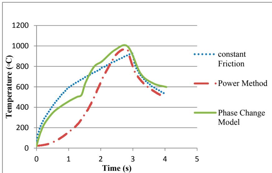
**Figure 14.** Comparison of the temperature profiles generated by constant friction method, power method, and phase change model.
