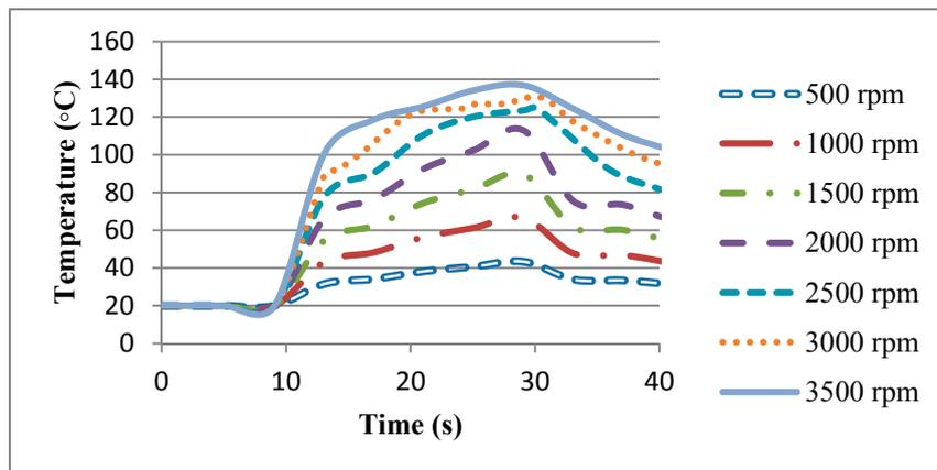
Figure 17. Temperature profiles generated by varying rotational speed.
