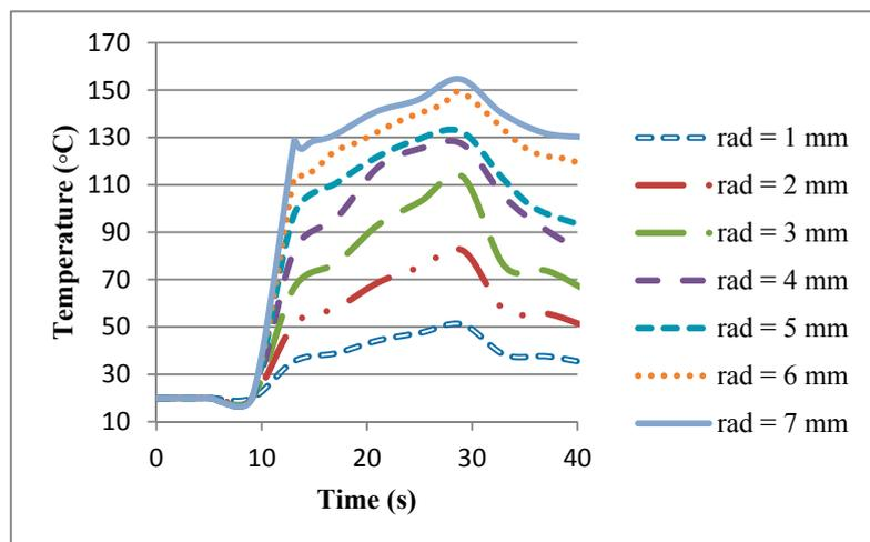
**Figure 15.** Temperature profiles generated by varying radius of the work-piece.
