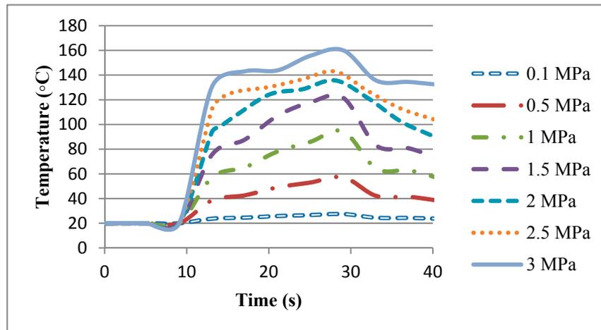
Figure 16. Temperature profiles generated by varying applied pressure.
