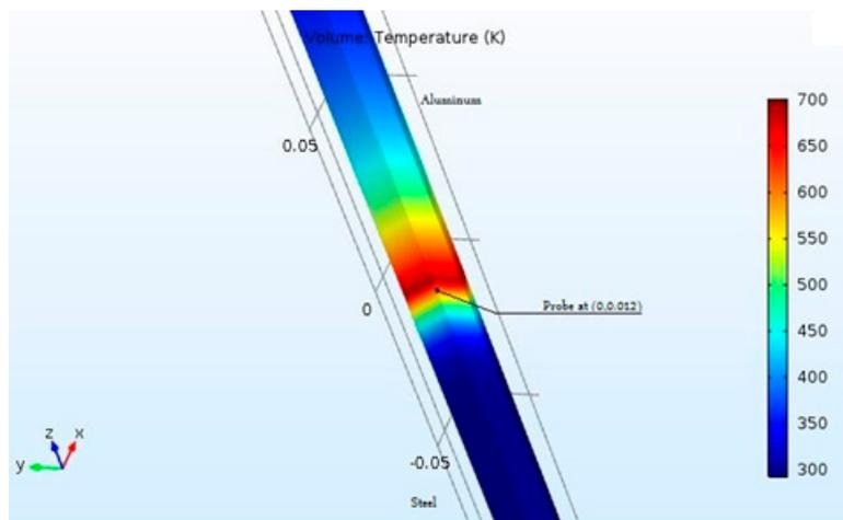
Figure 8. Temperature distribution for dissimilar metals.
