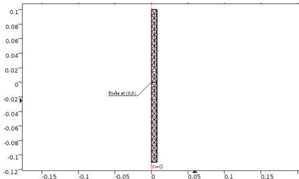
Figure 5. Geometry and its meshing.
