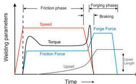
Figure 2. Variation of welding parameters with time in direct drive friction welding [1].
