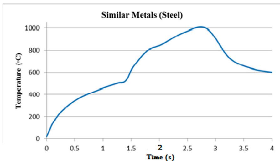
Figure 12. Temperature profile for the welding of similar metals.
