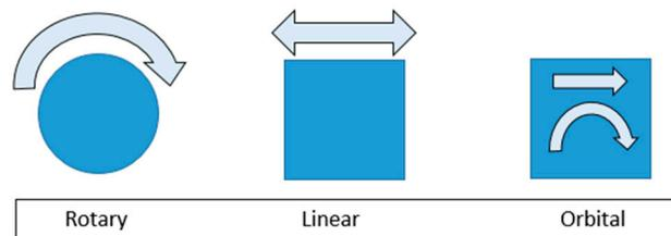
Figure 1. The three variants of the friction welding process [1].
