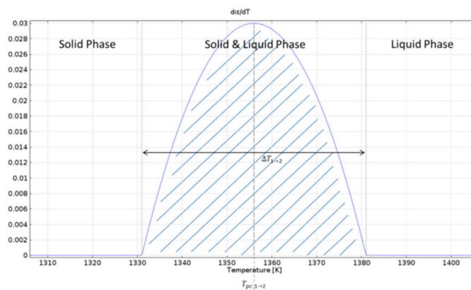
Figure 4. Plot example for  $d\alpha/dT$ —derivative of phase transition function [11].
