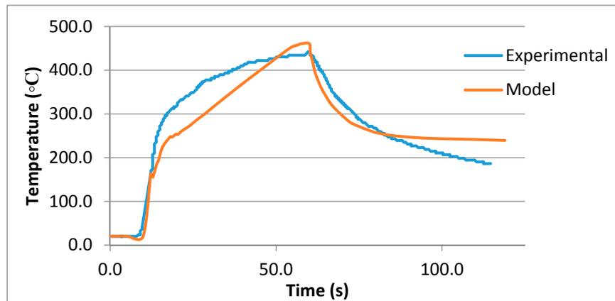
**Figure 13.** Comparison of experimental and model generated temperature profile for dissimilar metals.
