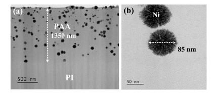
**Figure 10.** (**a**) Cross-sectional TEM images of the PI film after Ni reduction, followed by heat treatment in an oven at 85 °C for 5 min. (**b**) Enlarged image of the Ni nanoparticles embedded in the PAA layer.
