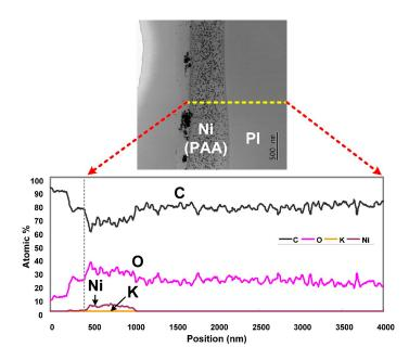
Figure 9. Elemental line-scan result across the surface sublayer of the PI film after Ni reduction.
