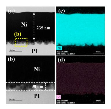
**Figure 4.** (**a**) Cross-sectional TEM image of the Ni-metallized PI film with the KOH concentration of base treatment of 0.5 M. (**b**) Enlarged image of the interfacial region marked in (**a**). (**c**,**d**) Elemental mapping results of Ni and P in the Ni-metallized PI film, respectively.
