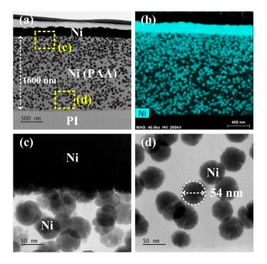
**Figure 5.** (**a**) Cross-sectional TEM image of the Ni-metallized PI film with a KOH base treatment concentration at 5.0 M. (**b**) Elemental mapping result of Ni in the Ni-metallized PI film. (**c**,**d**) Enlarged images of the interfacial and interior regions marked in (**a**).
