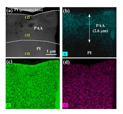
**Figure 6.** (a) Cross-sectional TEM image of the PI film after base treatment with a KOH concentration of 5.0 M. (**b**–**d**) Elemental mapping results of K, C, and O in the KOH-treated PI film, respectively.
