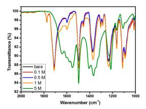
Figure 2. Transmittance spectra of the PI films before and after base treatment of KOH.
