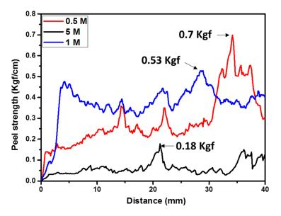
Figure 11. Peel strength of the electroless Ni layers on two PI films modified by 0.5 M and 5.0 M KOH.
