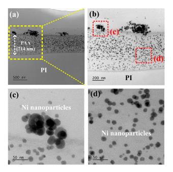
**Figure 8.** (**a**) Cross-sectional TEM image of the PI film after Ni reduction (The KOH concentration of base treatment is 5.0 M). (**b**) Enlarged image of the poly(amic acid) (PAA) layer marked in (**a**). (**c**,**d**) Enlarged images of the surface and interior regions of the PAA layer, respectively, marked in (**b**).
