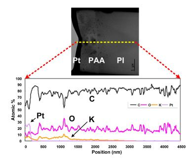
**Figure 7.** Elemental line-scan result across the surface sublayer of the PI film after base treatment of KOH.
