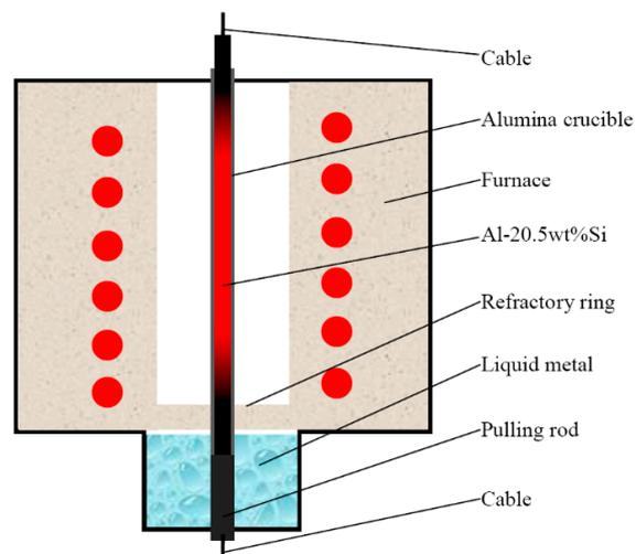
**Figure 1.** Schematic view of the solidification setup.
