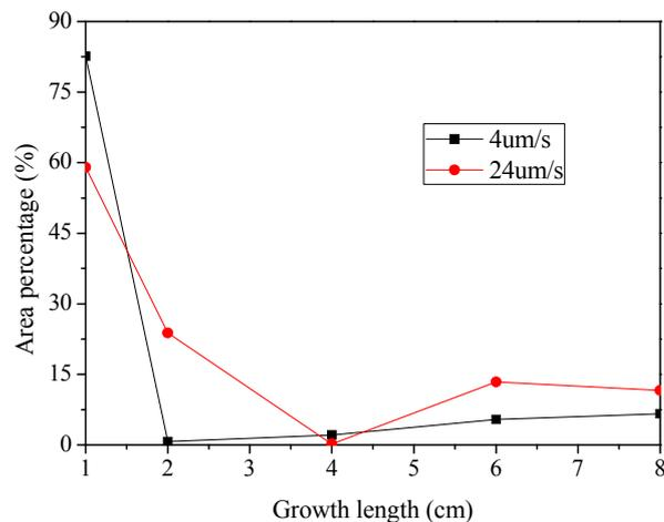
**Figure 5.** Measured area percentage of primary silicon in transversal sections of Al-Si hypereutectic alloy solidified at growth velocities of 4  $\mu\text{m/s}$  and 24  $\mu\text{m/s}$ .
