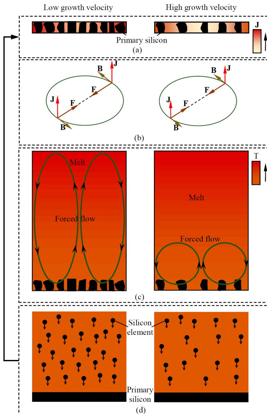
**Figure 6.** Schematic view of the primary silicon segregation mechanism under different growth velocities: (a) electric current density ( $J$ ) distribution; (b) induced magnetic intensity ( $B$ ) and Lorentz force ( $F$ ); (c) forced flow inside melt ( $T$ : temperature); (d) silicon element transportation for primary silicon precipitation.
