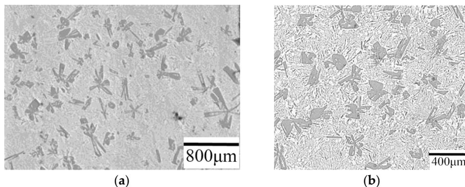
**Figure 3.** Micrographs in the different longitudinal sections of the original sucked sample at different zoom scales; (a) small; (b) large.
