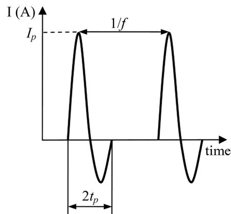
**Figure 2.** Waveform of the applied electric current pulse.
