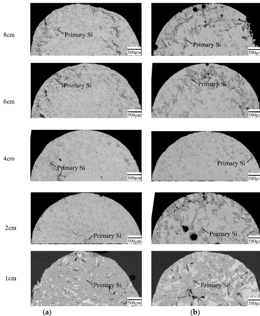
**Figure 4.** Solidified structure of Al-Si alloys with a conducted electric current pulse (ECP) on transversal sections at different growth lengths: (a)  $4 \mu\text{m/s}$ ; (b)  $24 \mu\text{m/s}$ .
