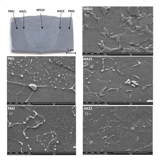
**Figure 3.** Structure of the material of components of the repair welded joint marked ZS1 made from 14MoV6-3 steel after 169,000 h service; microstructure investigation locations (**a**): parent material marked (**c**) PM1, (**e**) PM2; heat affected zone marked (**d**) HAZ1, (**f**) HAZ2; weld marked (**b**) WELD.
