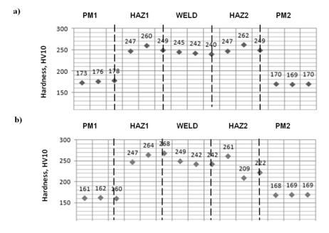
**Figure 5.** Distribution of the results of HV10 hardness measured on transverse microsections of the repair welded joint made from 14MoV6-3 steel. Test location—transverse microsection: (**a**) ZS1; (**b**) ZS2.
