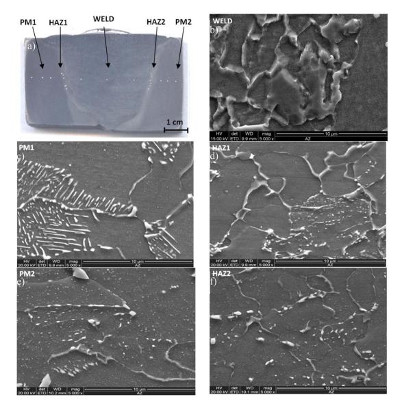
**Figure 4.** Structure of the material of components of the repair welded joint marked ZS2 made from 14MoV6-3 steel in the as-received condition and after 169,000 h service; investigation performance locations (**a**): parent material marked (**c**) PM1, (**e**) PM2; heat affected zone marked (**d**) HAZ1, (**f**) HAZ2; weld marked (**b**) WELD.
