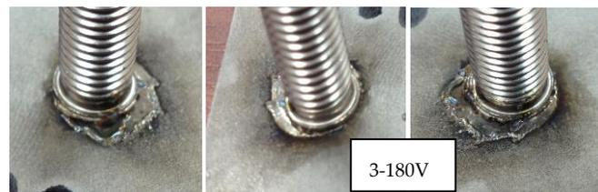
**Figure 8.** Visual inspection images of samples: 1-140 V, 2-160 V, and 3-180 V according to ISO 14555.
