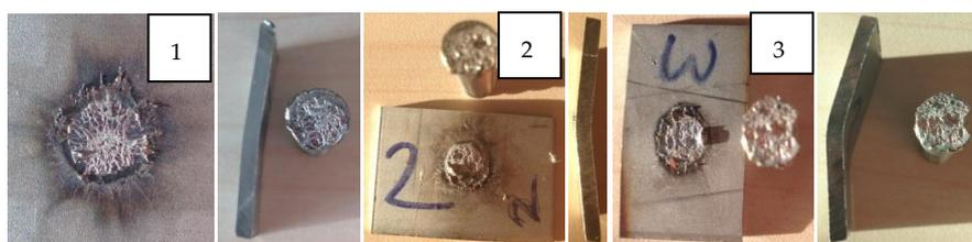
**Figure 14.** Macro images of split studs (1-140 V, 2-160 V, 3-180 V) and curvature of plates as examples.
