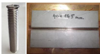
**Figure 3.** AISI 304 austenitic studs with S32205 Duplex plates.
