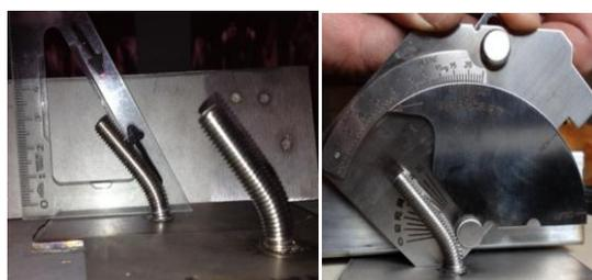
**Figure 13.** Bending angle determination of samples.
