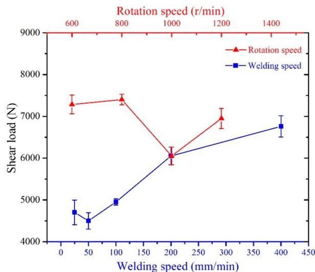
**Figure 17.** The variation of shear load with different welding parameters.
