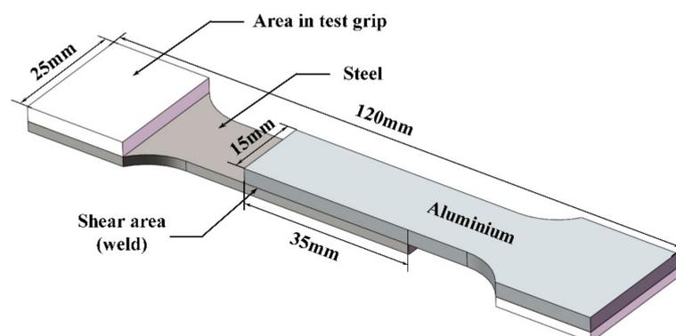
**Figure 2.** Dimensions of lap shear test sample.
