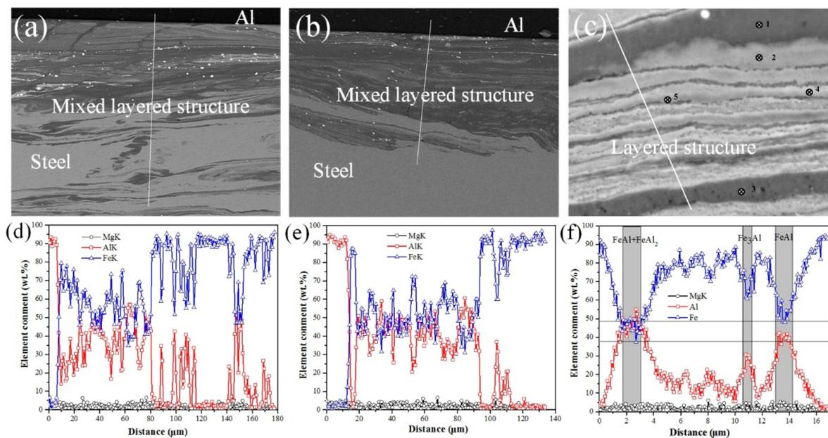
**Figure 11.** Scanning electron microscopy (SEM) line scanning results. (a) macrostructure of the interface at the center of the joint; (b) macrostructure of the interface on retreating side of the joint; (c) the layered structure at the interface; and (d–f) the line scan results.
