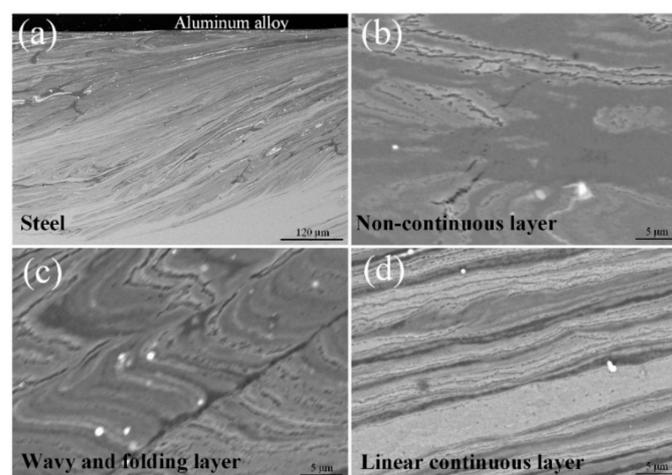
**Figure 9.** Interfacial macro- and microstructure of Al/steel lap joint with the rotation speed of 1200 rpm and welding speed of 200 mm/min. (a) Interfacial macrostructure; (b) non-continuous layer; (c) wavy and folding layer; and (d) linear continuous layer.
