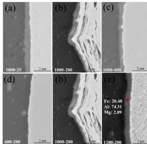
**Figure 13.** The variation of IMC thickness at the interface with different welding parameters. (a) 1000 rpm, 25 mm/min; (b) 1000 rpm, 200 mm/min; (c) 1000 rpm, 400 mm/min; (d) 600 rpm, 200 mm/min; and (e) 1200 rpm, 200 mm/min.
