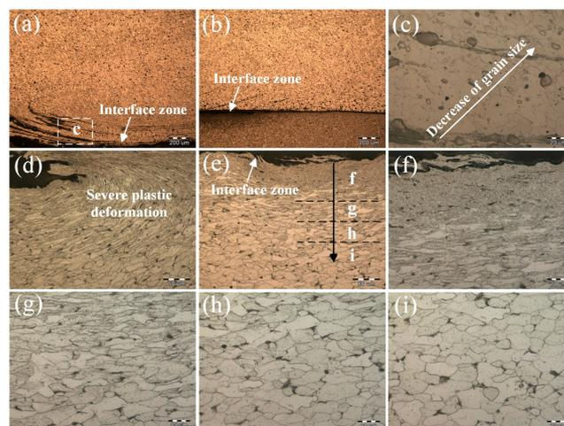
**Figure 5.** Interfacial microstructures of Al/steel lap joint with rotation speed of 1000 rpm and welding speed of 200 mm/min. (a–c) aluminum alloy side joint; (d) plastic deformed layer of steel side joint on retreating side; (e) plastic deformed layer of steel side joint in the center; and (f–i) higher magnifications shown in (e).
