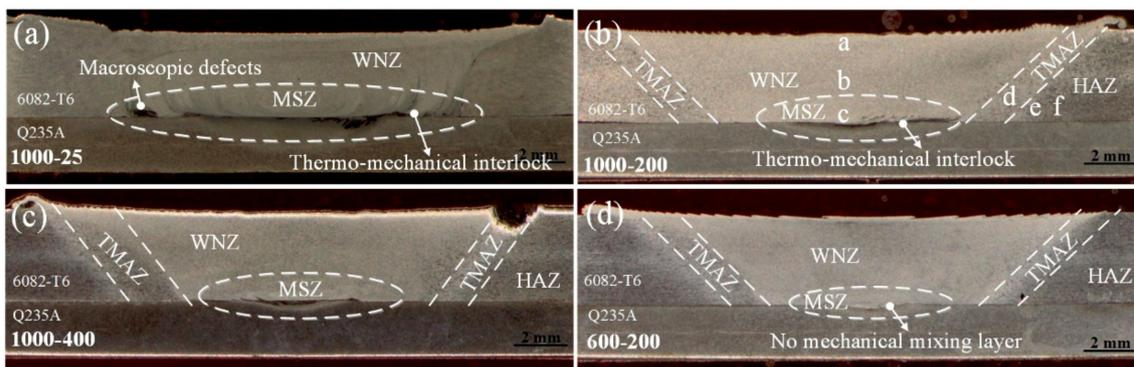
**Figure 3.** The comparison of macrostructure of Al/steel lap joint with different welding parameters. (a) 1000 rpm, 25 mm/min; (b) 1000 rpm, 200 mm/min; (c) 1000 rpm, 400 mm/min; and (d) 600 rpm, 200 mm/min.
