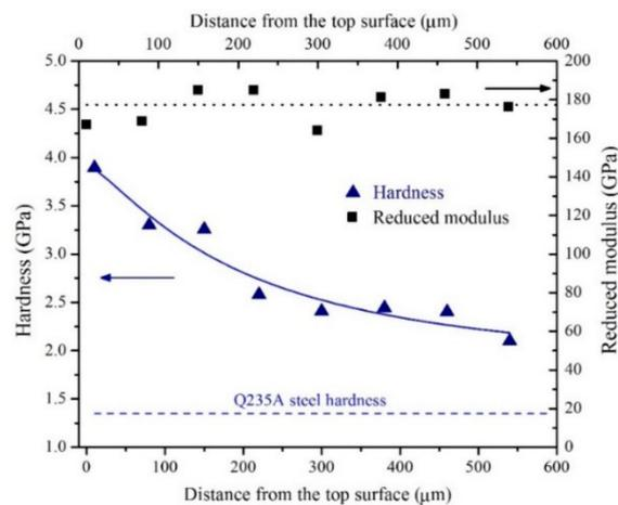
**Figure 15.** Variation of the nano-hardness and elastic moduli between the upper steel surface and steel base material.
