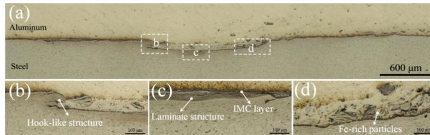
**Figure 7.** Interfacial macro-microstructures of Al/Fe lap joint with rotation speed of 1000 rpm and welding speed of 200 mm/min. (a) interfacial macrostructure; (b) hook-like feature; (c) laminate structure; and (d) particles composite-like structure.
