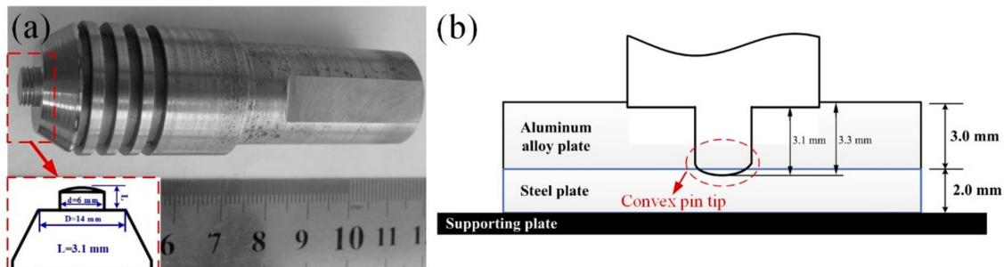
**Figure 1.** (a) The geometry shape and size of the designed tool; (b) the illustration of lap welding method.
