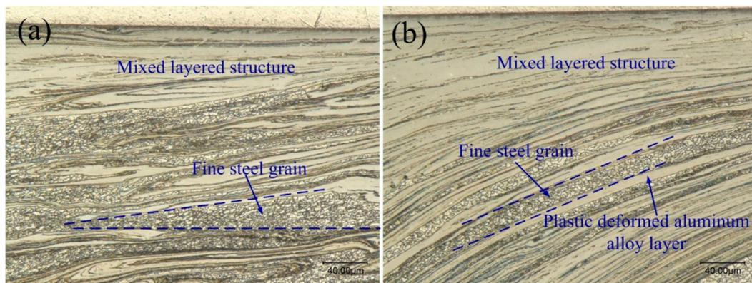
**Figure 10.** Mixed layered structure showing fine steel grain. (a) Middle part of interfacial zone; (b) advancing side of interfacial zone.
