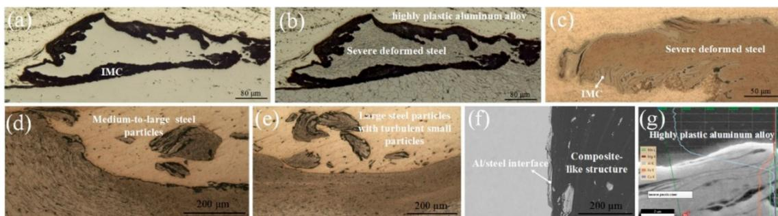
**Figure 8.** Detailed hook-like structure and composite-like structure of Al/steel lap joint. (a) Before corrosion; (b) after corrosion; (c) reaction between hook-like structure and severe plastic steel; (d) the steel particles; (e,f) large steel particles with turbulent small particles; and (g) IMCs formation at the weld interface.
