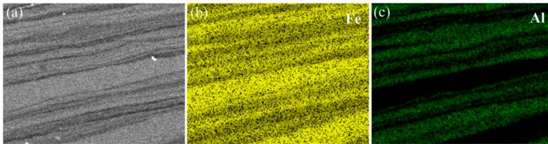
**Figure 12.** Chemical maps of the layered structure. (a) The composite map showing initial structure; (b) element Fe; and (c) element Al.
