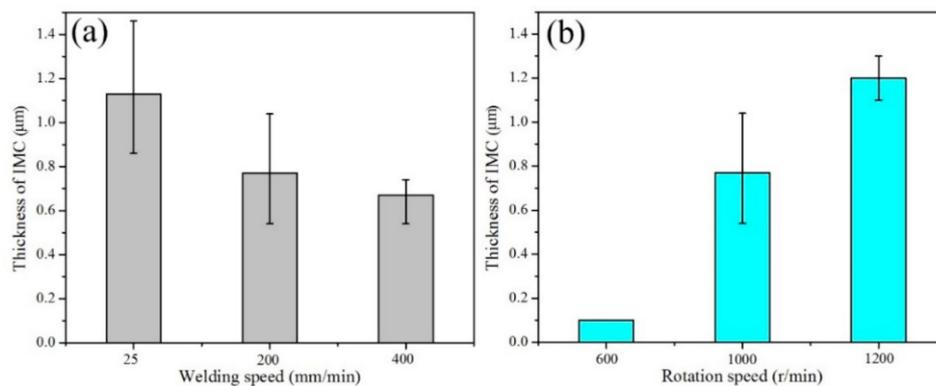
**Figure 14.** The variation of IMC thickness at the interface with different welding parameters. (a) Variation of the welding speed; and (b) variation of the rotation speed.
