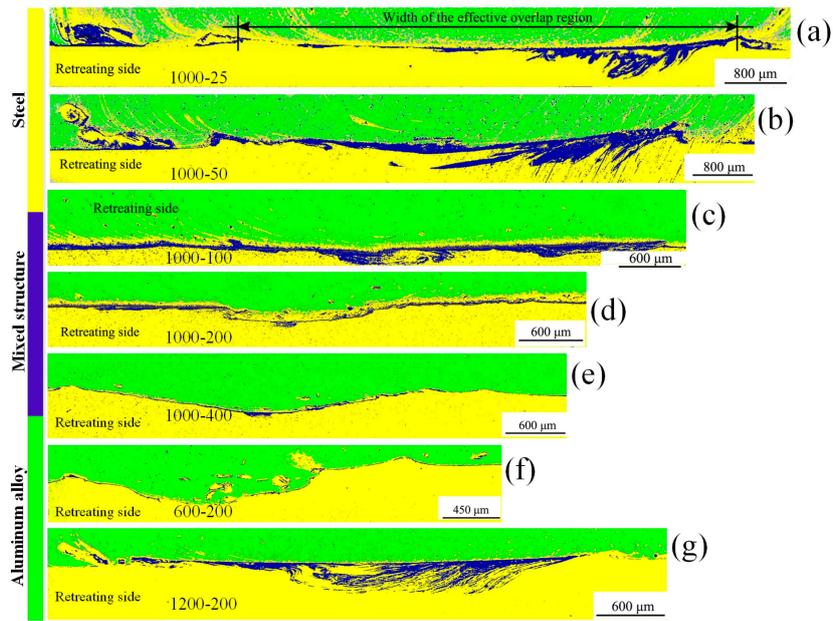
**Figure 4.** Macrographs of the joint interface showing distinctive interfacial features for weld made with different welding speeds and rotation speeds.
