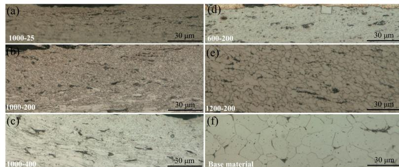
**Figure 6.** The variation of steel fine grain zone with different welding parameters. (a) 1000 rpm, 25 mm/min; (b) 1000 rpm, 200 mm/min; (c) 1000 rpm, 400 mm/min; (d) 600 rpm, 200 mm/min; (e) 1200 rpm, 200 mm/min; and (f) steel base material.
