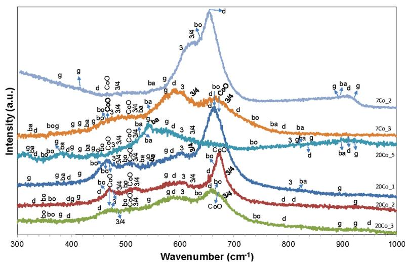
**Figure 11.** Representative Raman spectra from the surface of Al-7 wt.% Co and Al-20 wt.% Co, after cyclic polarization (3.5 wt.% NaCl, 25 °C). d: diaspore, b: boehmite, g: gibbsite, ba: bayerite, 3/4:  $\text{Co}_3\text{O}_4$ , 3: CoOOH.
