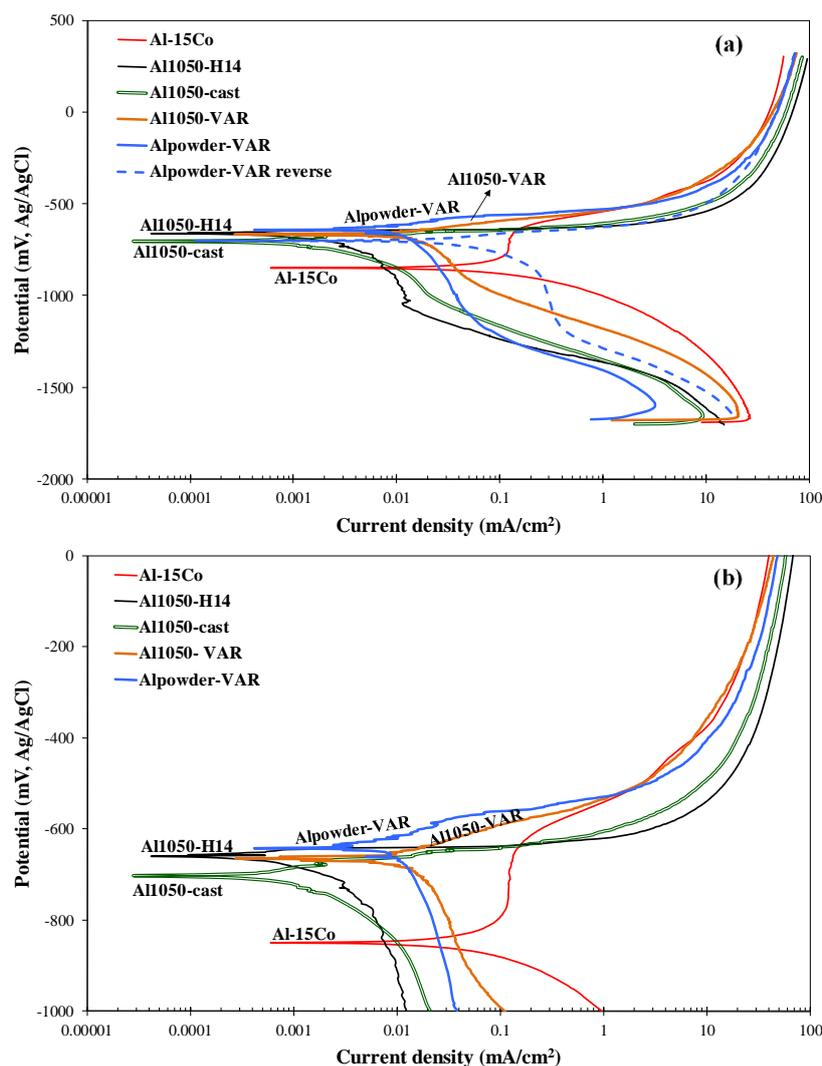
**Figure 5.** Potentiodynamic polarization performance of CP-Al produced by VAR of CP-Al powder (Alpowder-VAR), VAR of Al1050 sheet (Al1050-VAR), casting of Al1050 (Al1050-cast), cold rolling (Al1050-H14) and Al-15 wt.% Co produced by VAR (3.5 wt.% NaCl, 25 °C); (a) full view; (b) magnified view at a selected range of potentials.
