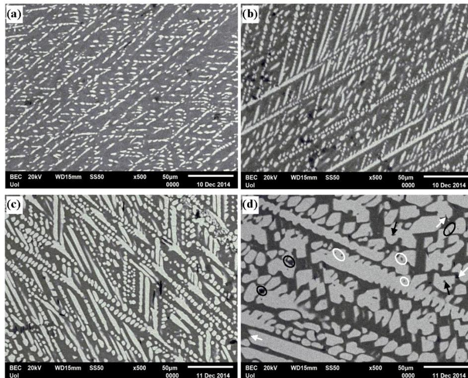
**Figure 2.** Microstructure of the alloys, as fabricated (BSE mode): (a) Al-7wt.% Co; (b) Al-10 wt.% Co; (c) Al-15 wt.% Co; (d) Al-20 wt.% Co; white outlined ellipses: pores at the intersections of dendrites and dendrite arms; black outlined ellipses: narrow and closed gaps in the matrix between  $\text{Al}_9\text{Co}_2$  particles; white arrows: pores, microdefects at sharp points of  $\text{Al}_9\text{Co}_2$  particles; black arrows: pores in the middle of  $\text{Al}_9\text{Co}_2$  phase.
