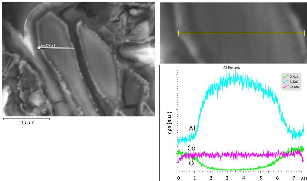
**Figure 9.** Cross-section (SE mode) of Al-15 wt.% Co after cyclic polarization (3.5 wt.% NaCl, 25 °C) and EDX line scan across a blade of  $\text{Al}_2\text{O}_3$ .
