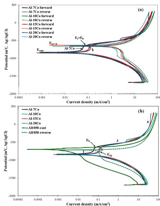
**Figure 4.** Potentiodynamic polarization behavior of the various alloys and CP-Al fabricated by casting of Al1050 sheet (Al1050-cast) in 3.5 wt.% NaCl, at 25 °C. (a) Al-Co cyclic polarization; (b) Al-Co forward polarization and CP-Al cast cyclic polarization.
