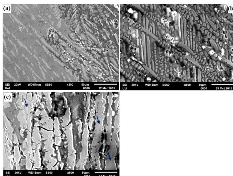
**Figure 6.** Cross sections (SE mode) of (a) Al-7 wt.% Co, (b) Al-15 wt.% Co and (c) Al-20 wt.% Co after cyclic polarization (3.5 wt.% NaCl, 25 °C); the blue arrows in Figure 6c point at the  $\text{Al}_{13}\text{Co}_4$  phase.
