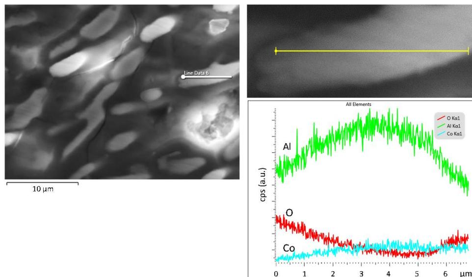
**Figure 8.** Cross-section (SE mode) of Al-7 wt.% Co after cyclic polarization (3.5 wt.% NaCl, 25 °C) and EDX line scan across a plate of  $Al_2O_3$ .
