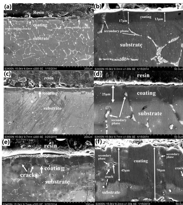
**Figure 5.** SEM cross-sectional morphologies of the coated samples at low and high magnification. (a) and (b) are 160 °C-coated sample; (c) and (d) are 170 °C-coated sample; (e) and (f) are 180 °C-coated sample.
