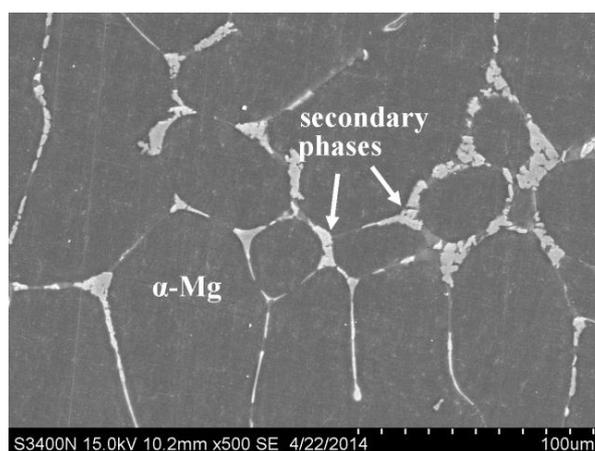
**Figure 1.** Microstructure of the Mg alloy.
