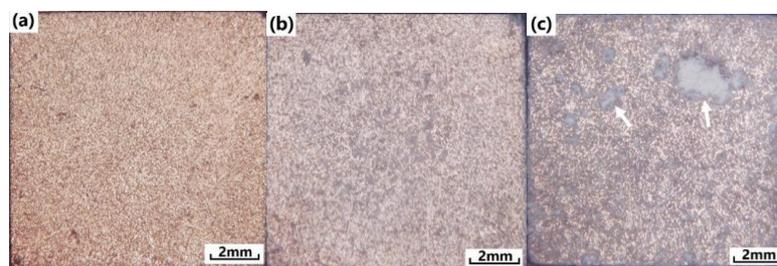
**Figure 3.** Macro morphologies of the coated samples. (a) 160 °C-coated; (b) 170 °C-coated; (c) 180 °C-coated.
