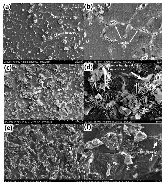
**Figure 4.** SEM surface morphologies of the coated samples at low and high magnification. (a) and (b) are 160 °C-coated sample; (c) and (d) are 170 °C-coated sample; (e) and (f) are 180 °C-coated sample.
