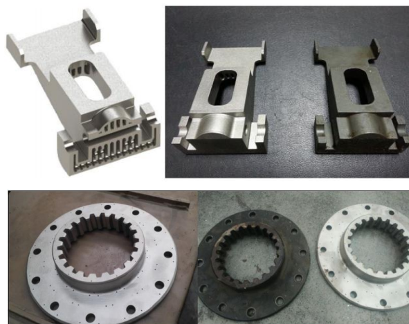
Figure 28. Final redesigned stopper ( up ) and connecting plate ( down ) with original parts.
