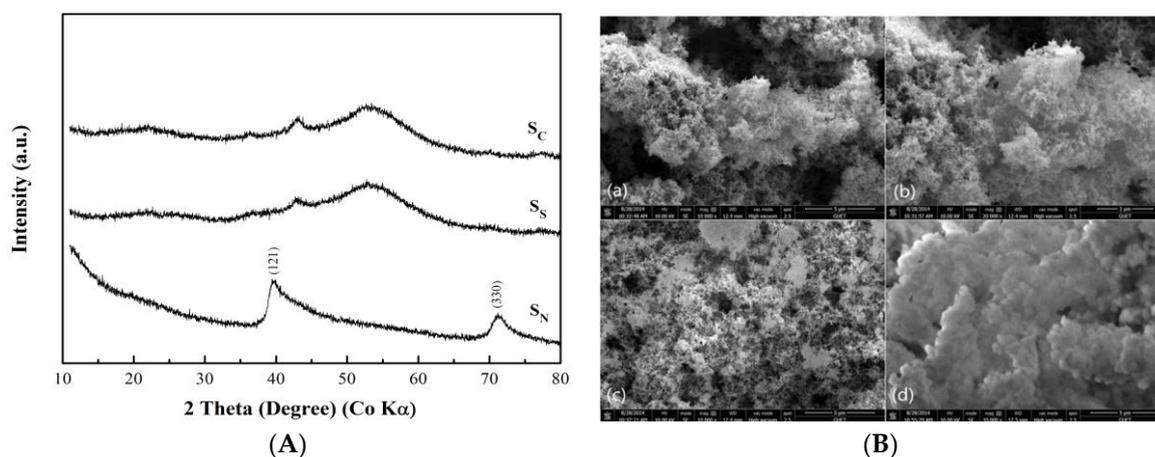
**Figure 1.** (A) XRD patterns and (B) SEM micrographs of the as-prepared Co-B alloys: (a) and (b) for  $S_C$  at different magnifications; (c) for  $S_S$ ; and (d) for  $S_N$ .
