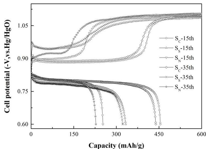
**Figure 3.** Potential-capacity curves of Co-B alloy anodes at the 15th and 35th cycles.
