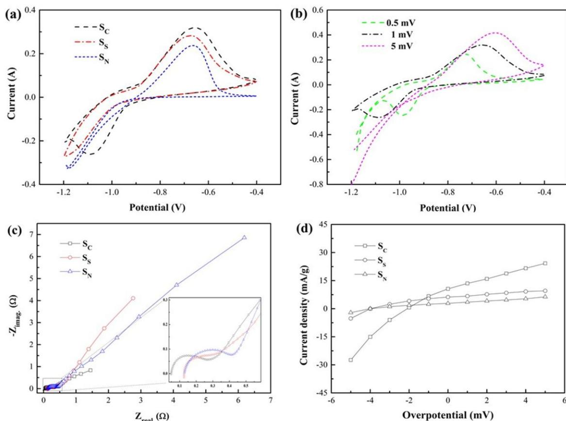
**Figure 4.** Typical CV curves of Co-B alloys: (a) the scanning rate was 1 mV/s; (b) the CV curves of the S<sub>C</sub> at different scanning rates; (c) EIS and (d) LP of Co-B alloy electrodes at 50% DOD and 298 K.
