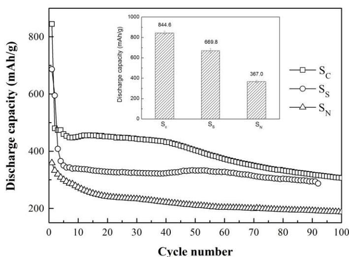
**Figure 2.** Cycling life of Co-B alloys as the anodes. The inset shows the maximum discharge capacity.
