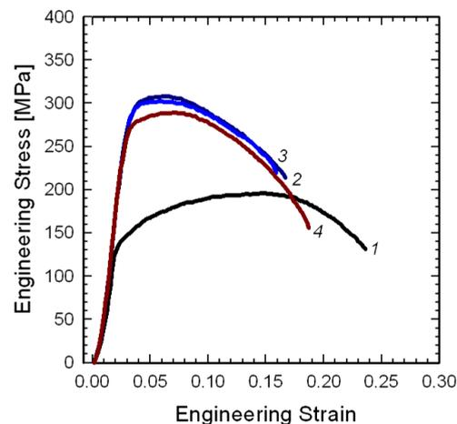
**Figure 4.** Typical engineering stress—engineering strain curves from tensile testing of the Al 6101 alloy (1) in the T1 condition; (2) after ECAP-C processing; (3) after ECAP-C processing and AA at 170 °C for 12 h; and (4) after ECAP-C processing and AA at 190 °C for 6 h.
