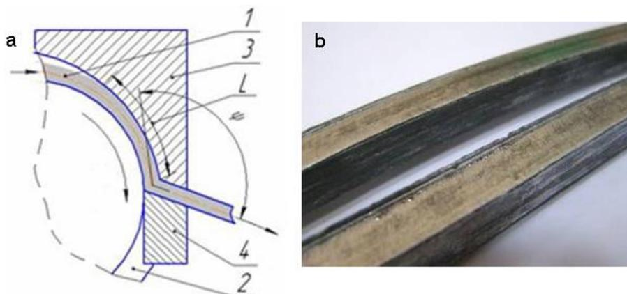
**Figure 1.** (a) A schematic illustration of ECAP-C machine: 1—ingot; 2—running wheel die; 3—pressure arrangement working surface; 4—a gauge;  $\psi$ —angle of intersection with a wheel die;  $L$ —arc of a rod grip; and (b) the surface of wire rods of Al 6101 alloy after six cycles of ECAP-C at  $130$  °C.
