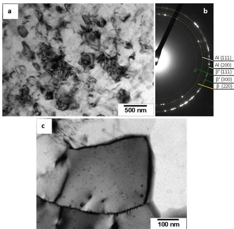
**Figure 3.** (a) Microstructure and (b) SAED patterns of the Al 6101 alloy after ECAP-C; and (c) view of strengthening second-phase precipitates formed in the matrix of the Al alloy after ECAP-C processing.
