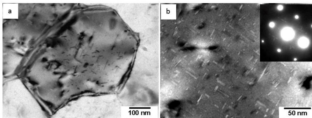
**Figure 6.** Strengthening second-phase precipitates present in the Al matrix of the ECAP-C processed alloy artificially aged at 170 °C for 12 h: (a) bright field TEM image; and (b) bright field TEM image and corresponding SAED patterns (the crystal is close to the [001] zone axis orientation).
