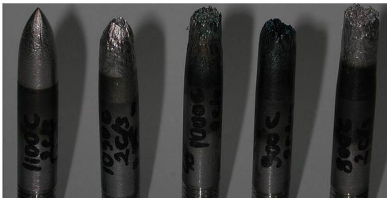
**Figure 3.** Some of the broken pieces of specimens after hot tensile tests.
