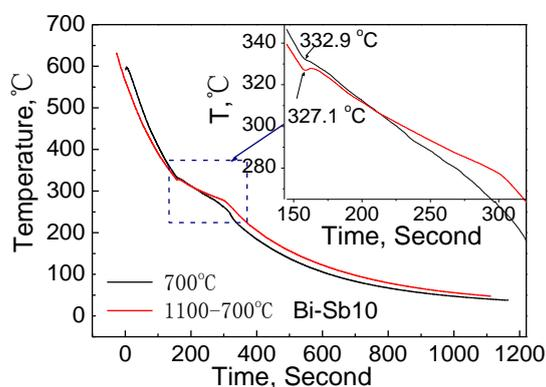
**Figure 17.** Bi-Sb10 T-t curves of different melts.
