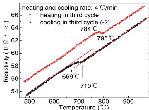
**Figure 11.**  $\rho$ - $T$  curves of Sn-Sb5wt% melt.
