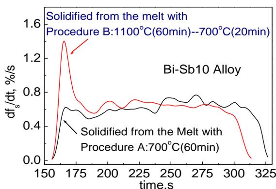
**Figure 18.** Solidification rate obtained by NTA method.
