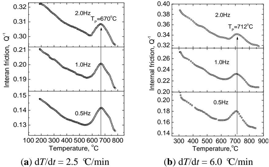
**Figure 1.** Internal friction behavior of the melt Pb-Sn61.9.
