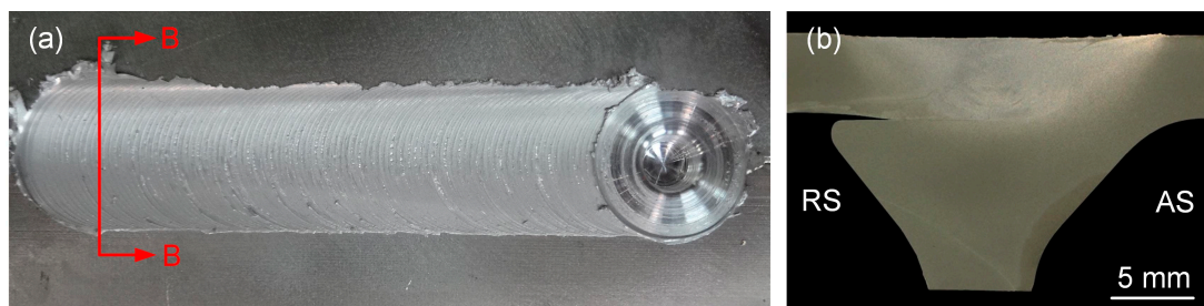
Figure 13. The obtained joint: (a) surface appearance, (b) cross-section of B-B in (a).
