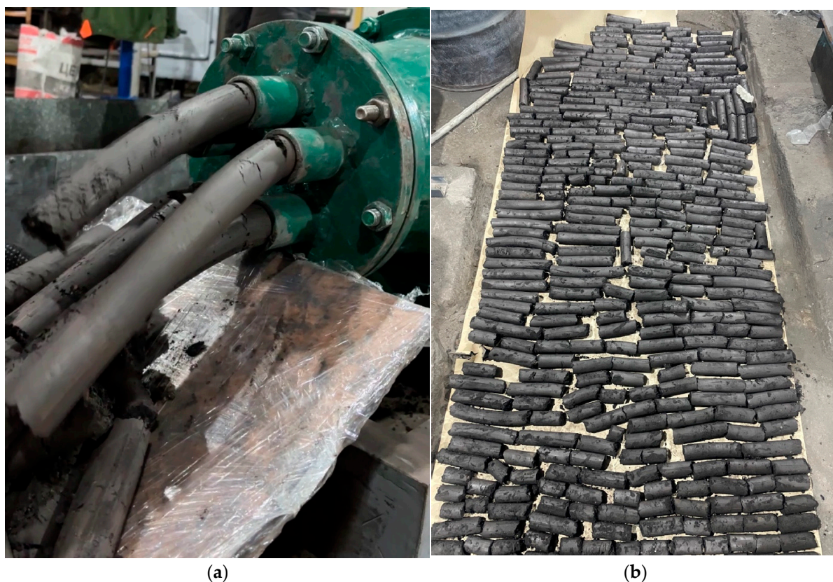
Figure 6. Fragment of the produced briquette batch: (a) briquette output; (b) finished briquettes.
