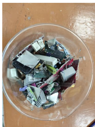
Figure 1. Photograph of the fragmented PCB material used as the working electrode.
