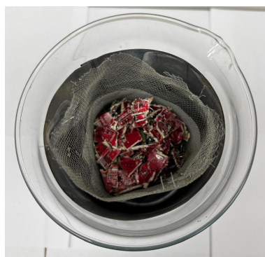
Figure 2. Photograph illustrating the configuration of the anodic basket and membrane used in the electrochemical leaching experiments.
