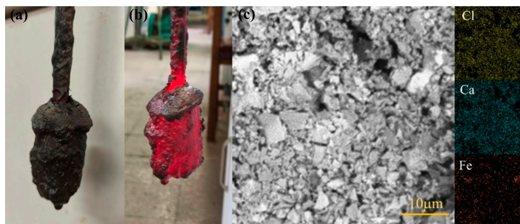
Figure 10. (a) Cooled output product (b) High-temperature output product after exiting salt melt (c) SEM analysis of cathode output product (Image courtesy of H. Aghajani).
