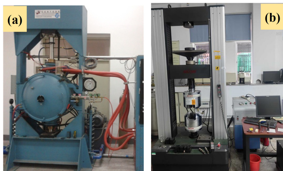
Figure 2. HP 12 × 12 × 12 Vacuum Hot Press Furnace (manufactured by CENTORR Vacuum Industries, Nashua, NH, USA) (a) and CMT5105 Electronic universal testing machine (Shenzhen SANS Testing Machine Co., Ltd., Shenzhen, China) (b).
