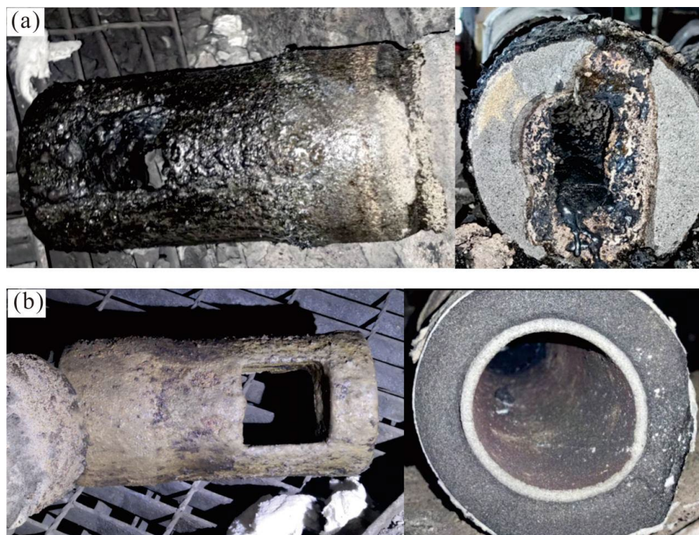
Figure 6. Submerged entry nozzle morphology after casting: (a) conventional weir–dam strand; (b) filter-equipped strand.
