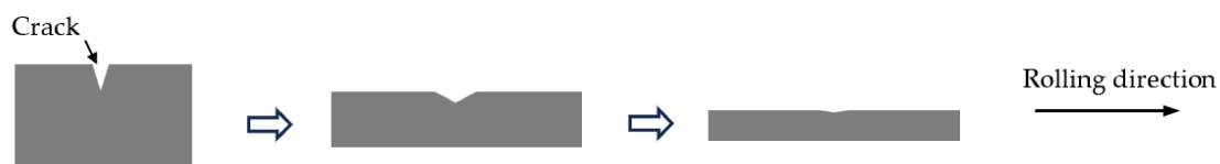
Figure 7. Schematic diagram showing expected improvement of the cracks in the width direction after rolling.
