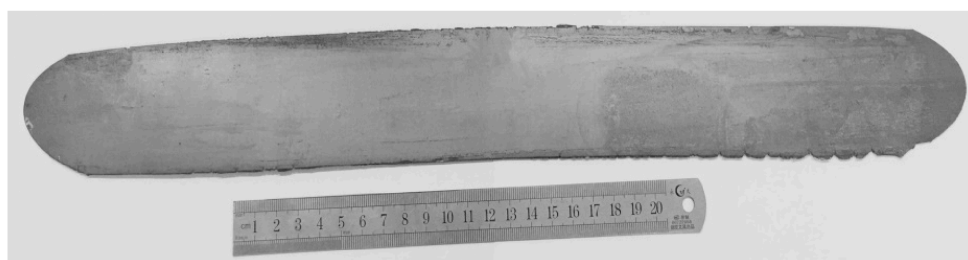
Figure 1. Macroscopic morphology of the CoCrFeNiAl 0.5 Ti 0.1 HEA sheet.
