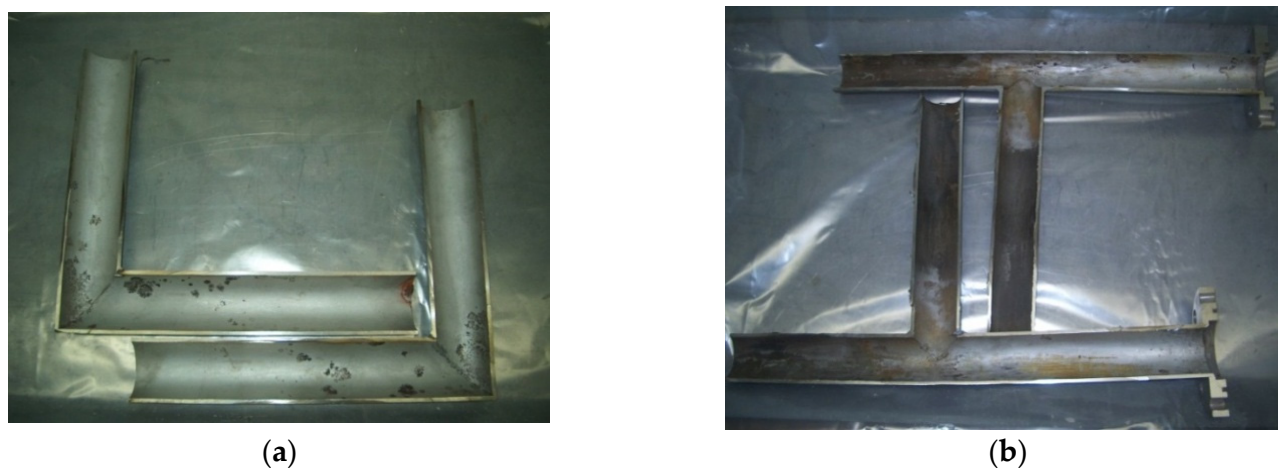
Figure 2. External view of the studied chlorinator elements: (a) section located at the cooler position; (b) section located at the heater position.
