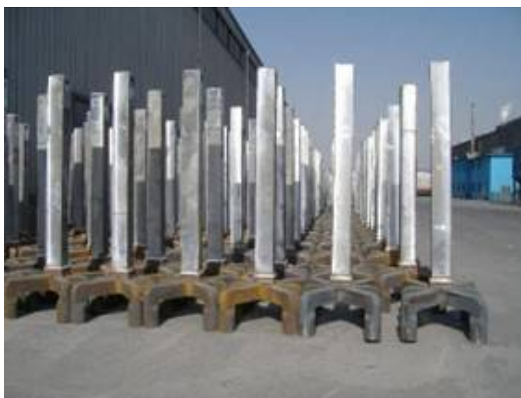
Figure 18. Final anode steel claw.
