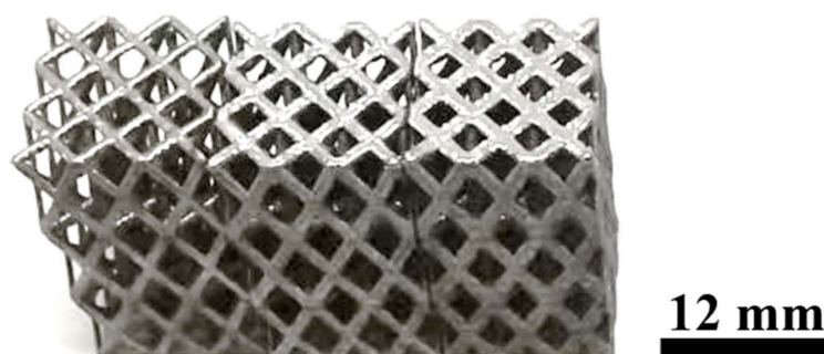
Figure 4. Actual FCC lattice structure specimens with 0.6 mm, 0.8 mm, and 1.0 mm strut diameter.
