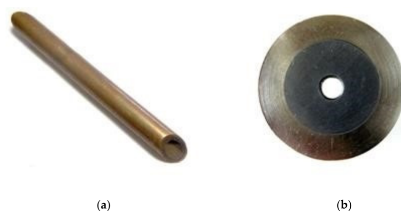
Figure 16. Experimental products using MPC: (a)—a copper tube with inner powder coating (outer diameter 18 mm, length 300 mm); (b)—a cross-section of a two-layered part with an inner piece of WC-Co alloy and an external frame of Fe-C-Cu alloy.
