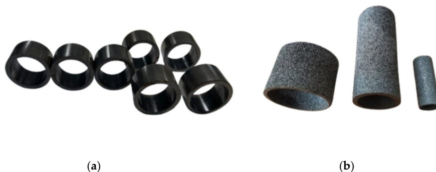
Figure 5. Parts produced from (a) Fe-C powder composition (residual porosity 5–10%) and (b) titanium powder-based (residual porosity 15–30%) using the MPC technique.
