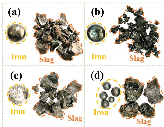
Figure 6. Macroscopic morphology of slag and iron separation after smelting under different \text{MgO} dosage. (a) 0%; (b) 5%; (c) 10%; (d) 15%.
