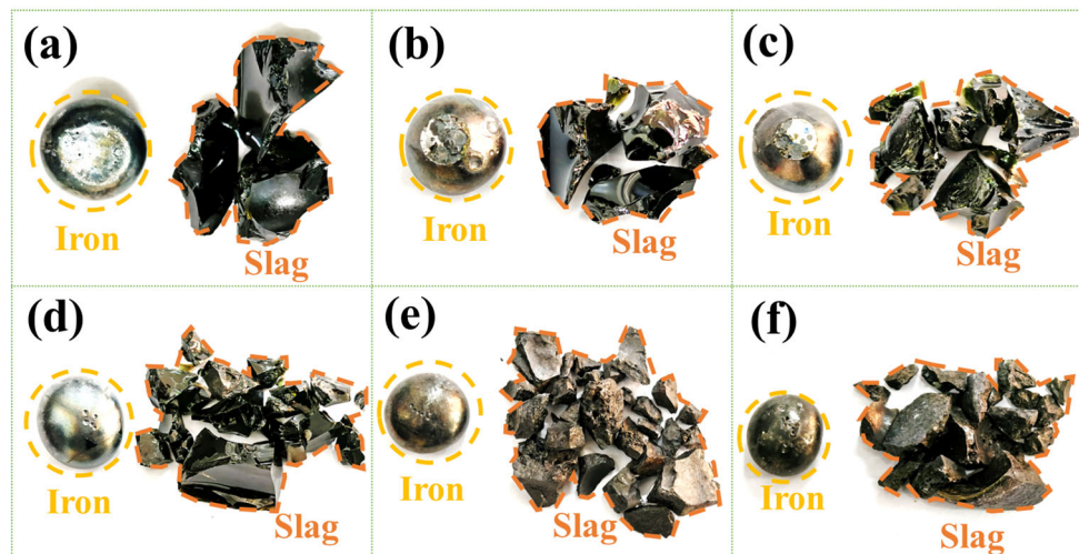
Figure 4. Macroscopic morphology of slag and iron separation after smelting under different basicity conditions. (a) R = 0.035 ; (b) R = 0.5 ; (c) R = 1.0 ; (d) R = 1.5 ; (e) R = 2.0 ; (f) R = 2.5 .
